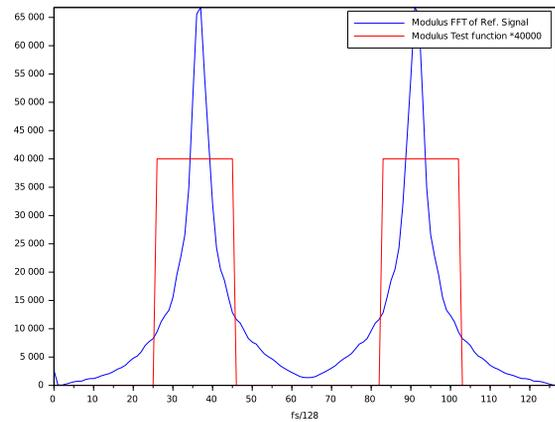
Figure 3: FFT (modulus) of the beam pulses and response of the test function (multiplied by 40000 to make it visible).
