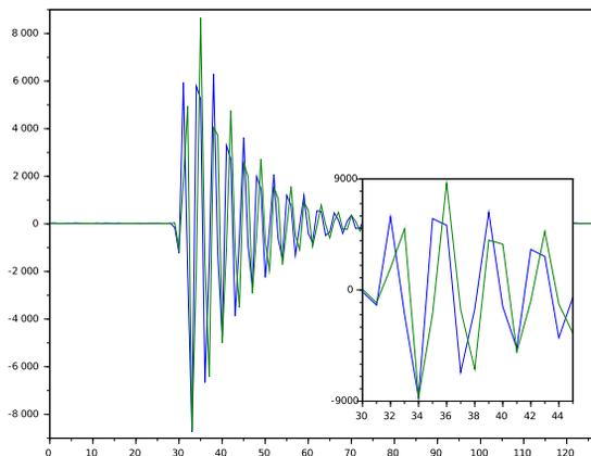
Figure 2: Reference signal of two beam pulses with unlocked ADC and LO. The sub-plot zooms to samples #30 – 45.
