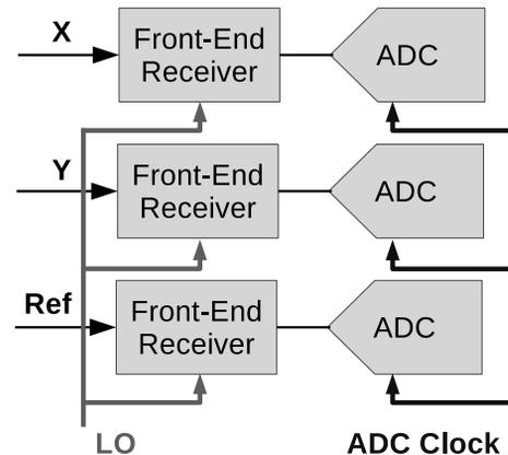
Figure 1: Cavity BPM receiver hardware block diagram.
