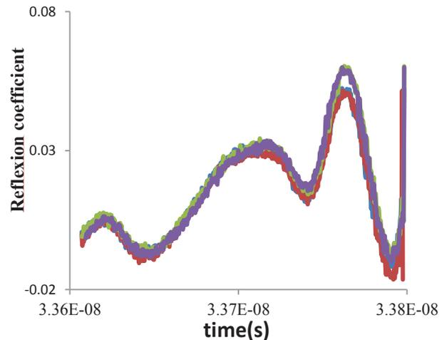
Figure: New BPM electrodes TDR responses.
