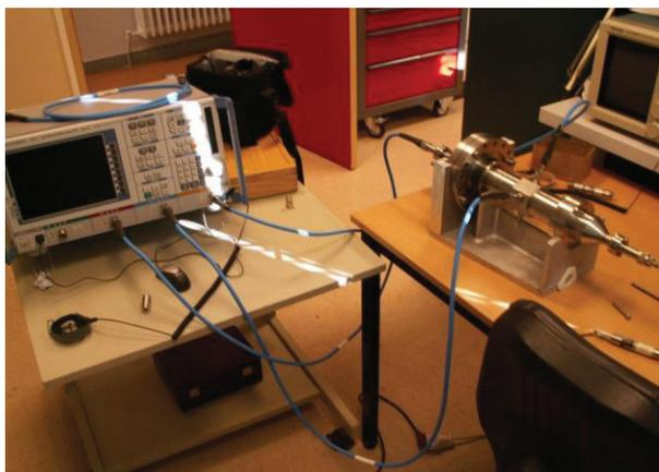
Figure 4: BPM current sensitivity measurement setup.
