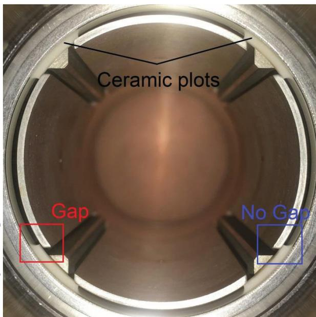
Figure 3: BPM with anti-gazing ceramic plots.
