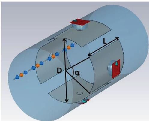
Figure 1 : Generic example of electrostatic BPM.
