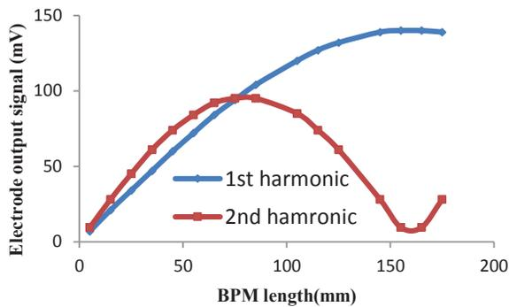
Figure 2: BPM simulations (beam current=5mA, centered beam,  $\beta=0.08$ ).
