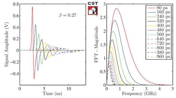
Figure 4: The legend shows the bunch length  $\sigma_b$  and the plotted signals represent output voltage from a single port in time (left) and frequency (right) domains for  $\beta = 0.27$ .
