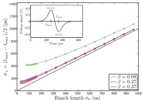
Figure 8: The relationship between the bunch length  $\sigma_b$  and the length of the pickup signal  $\sigma_s$  extracted from the time difference between the minimum and the maximum values of the pickup signal.
