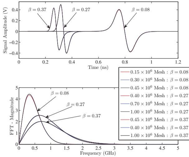
Figure 2: BPM output voltage from a single port in time (up) and frequency (down) domains versus mesh size. The beam parameter are  $\beta = 0.08, 0.27$  and  $0.37$ ,  $\sigma = 150$  ps, 1 nC bunch charge.
