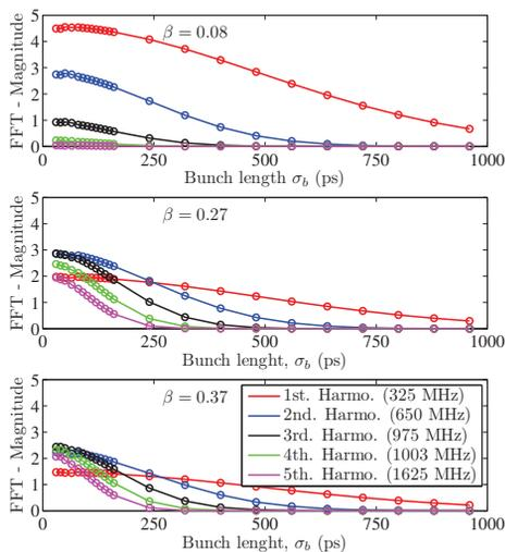
Figure 7: The Fourier components of the pickup signals at five harmonics of the bunching frequency versus bunch length.
