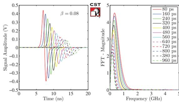
Figure 3: The legend shows the bunch length  $\sigma_b$  and the plotted signals represent output voltage from a single port in time (left) and frequency (right) domains for  $\beta = 0.08$ .
