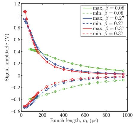
Figure 6: The change in the maximum and the minimum values of the pickup signal versus bunch length  $\sigma_b$ .
