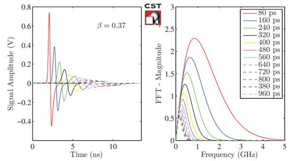
Figure 5: The legend shows the bunch length  $\sigma_b$  and the plotted signals represent output voltage from a single port in time (left) and frequency (right) domains for  $\beta = 0.37$ .
