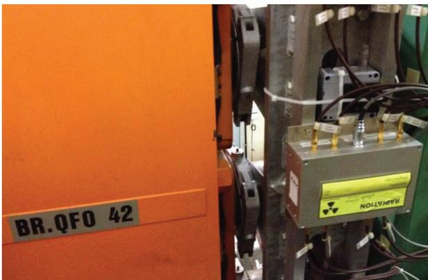
Figure 6: Dosimeter and electronics location.
