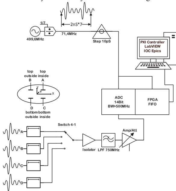
Figure 1: Block diagram of the bunch-resolved BPM system.
