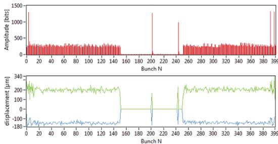
Figure 4: Fillpattern (over) and positions (under) of all filling bunches at BESSY II storage ring.
