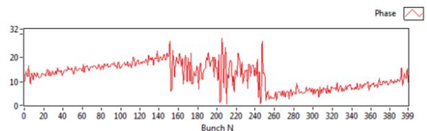
Figure 2: Longitudinal phase in units of 10 ps for a multi bunch fill induced by the gap at BESSY.
