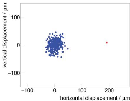
Figure 5: Spatial separation of individual bunches (PPRE bunch is marked in red) in low alpha mode at BESSY II.
