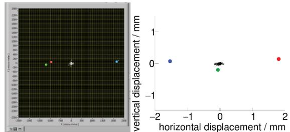
Figure 6: Orbit separation with 3 islands mode at BESSY II (left) and MLS (right). Both machines were operated with a homogenous fill pattern in the core beam, where one bunch was transferred to a single island [5]. The displacement of the stable, closed orbit of the island bucket was measured for the first turn (red), the second turn (green) and the third turn (blue).
