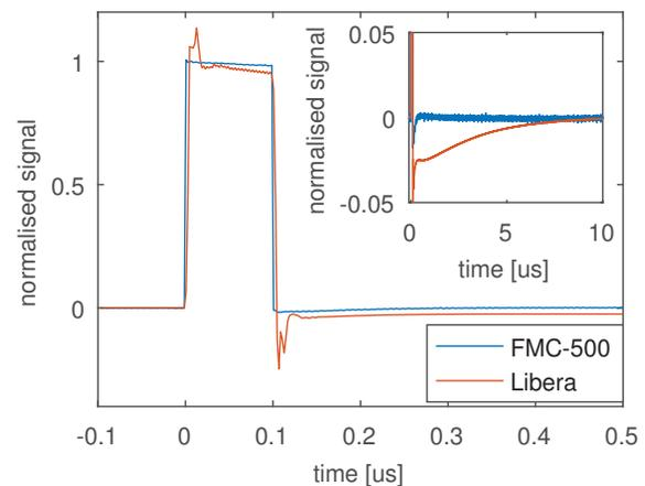
Figure 6: Normalised time response to a 100 ns pulse. Main graph shows pulse detail, while inset shows longer term settling.
