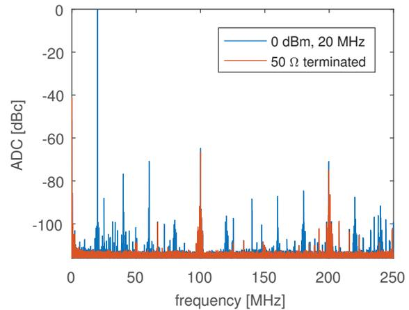
Figure 5: Spectrum with and without a 0 dBm 20 MHz tone (filtered by a crystal to remove harmonics from the generator). Fast Fourier Transform of  $2^{25}$  points.
