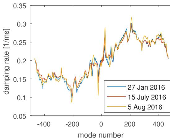
Figure 3: Damping rates of all longitudinal CBI.
