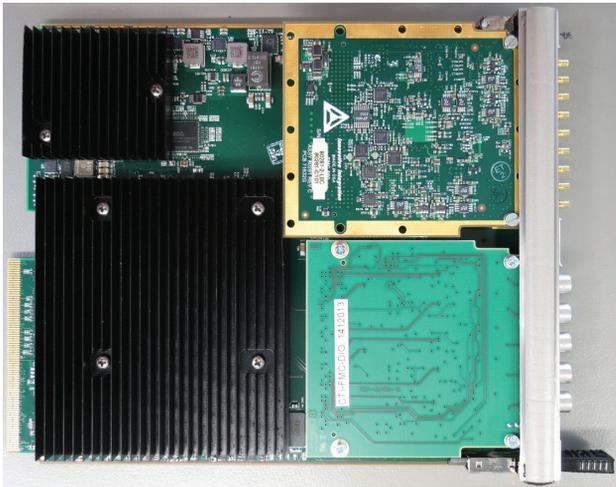
Figure 4: Photo of the assembly of FMC-500 (top right) and FMC-DIO-5Ch-TTL-A (bottom right) on the AMC525. Dimensions are 180 mm by 150 mm.
