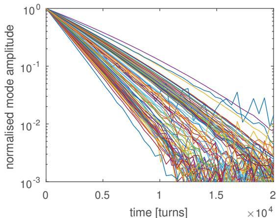
Figure 2: Normalised magnitude during damping of longitudinal CBI after excitation. Only every tenth mode of the total of 936 is shown for clarity.
