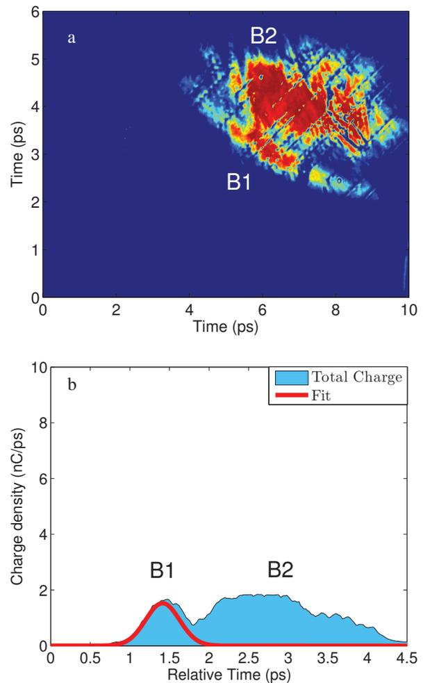
Figure 4: (a) Signature of the escaping electrons from target. The emitted charges are, respectively, 1.2 nC (B1) and 3 nC (B2). The gaussian envelopes represent the extrapolated charge profiles of each bunch. (b) Corresponding longitudinal charge profiles.
