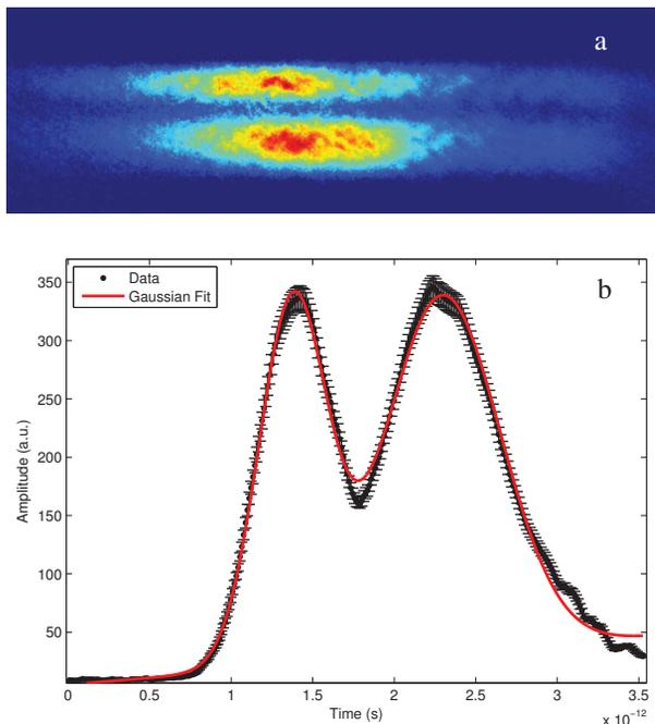
Figure 1: (a) Electro-optic signal of a comb-like bunch obtained with a 100  $\mu\text{m}$ -thick GaP crystal. (b) Corresponding temporal profile obtained by projecting the signal in (a).
