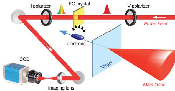
Figure 3: Setup of the experiment. The FLAME laser is focused on a metallic target that ejects electrons. The EOS diagnostics, based on a ZnTe crystal located 1 mm downstream the target, measures the temporal profile of the emitted electrons by means of an ultra-short probe laser.
