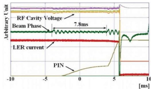
Figure 6: Loss monitor abort with beam phase oscillation.
