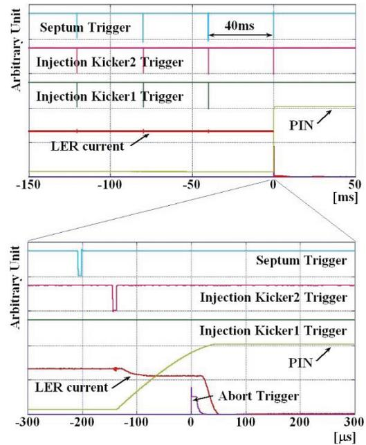
Figure 5: Beam loss that synchronized for injection timing.
