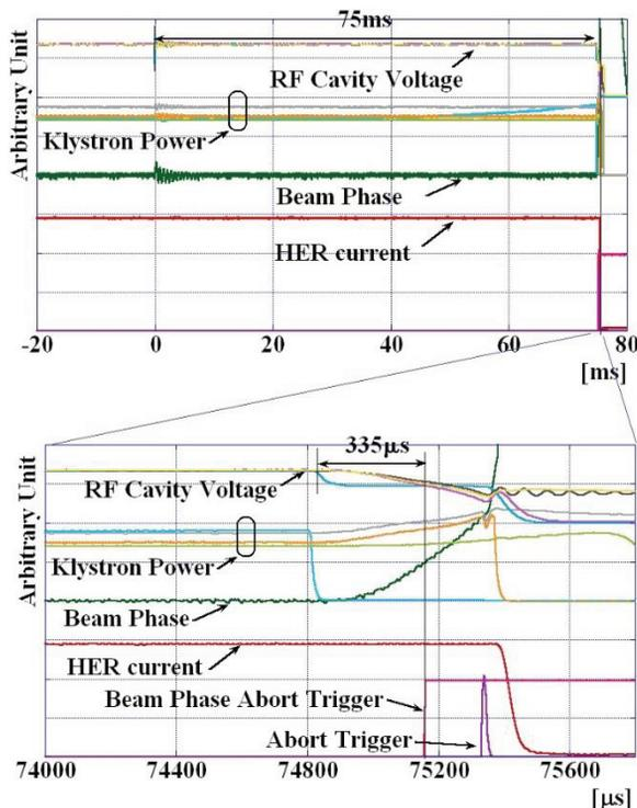
Figure 7: Beam phase abort caused by RF down.
