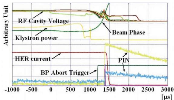
Figure 8: BP abort caused by earthquake.
