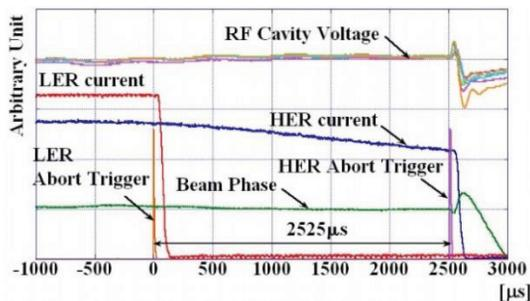
Figure 4: Loss monitor abort caused by HER beam loss.
