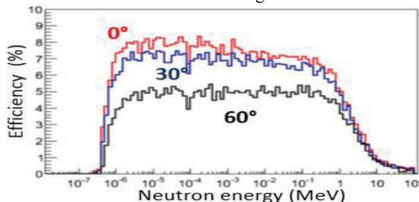
Figure 8: nBLM angular response to neutrons.
