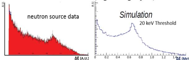
Figure 9:  $^{252}\text{Cf}$  data and simulation obtain by a Micromegas detector and sets of moderators.
