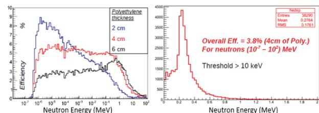
Figure 4: Neutron efficiency for 2, 4 and 6 cm moderator thickness (left) and the detected neutron spectrum for 4 cm thickness of polyethylene (right).
