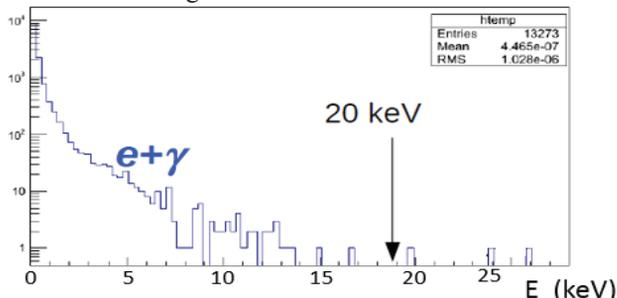
Figure 5:  $e^-$  and  $\gamma$  by-products of  $n+^{10}\text{B}$  reaction.
