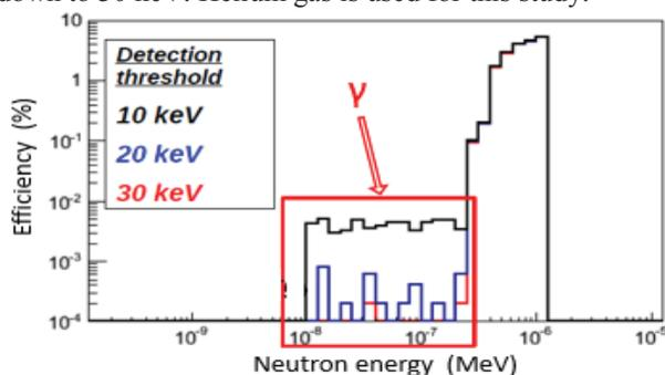
Figure 6: Thermal neutron efficiency for 4 cm moderator thickness.  $\gamma$  decays from Cd and  $^{10}\text{B}$  are highlighted in red.
