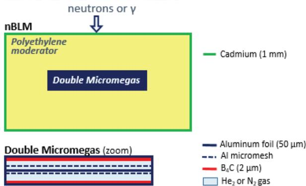
Figure 2: nBLM structure with a zoom on the double Micromegas. Overall size of such a monitor is about  $22 \times 22 \times 10\text{ cm}^3$ .
