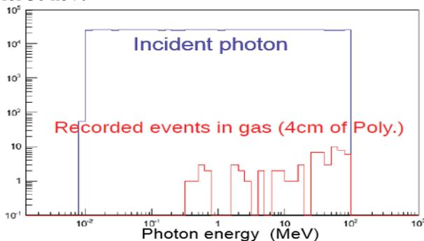
Figure 7: Incident photons (blue) and detected ones (red) for an nBLM integrating 4 cm moderator and He gas.
