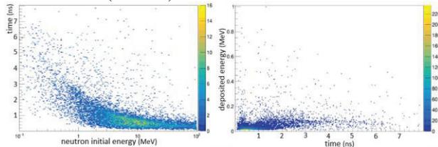
Figure 11: Time response for the fast Micromegas versus incident and deposited neutron energies.
