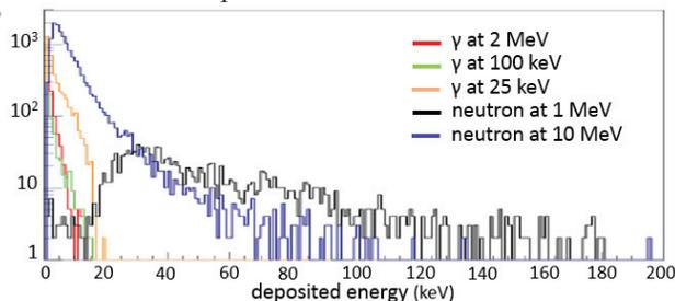
Figure 12: Fast Micromegas neutron and  $\gamma$  responses.
