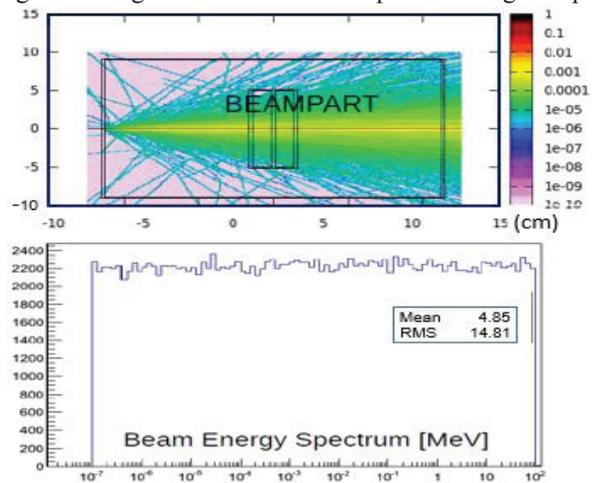
Figure 3: Neutron impacting on nBLM (2 cm moderator thickness) as seen by FLUKA (top) and the flat neutron double exponential energy spectrum (bottom).
