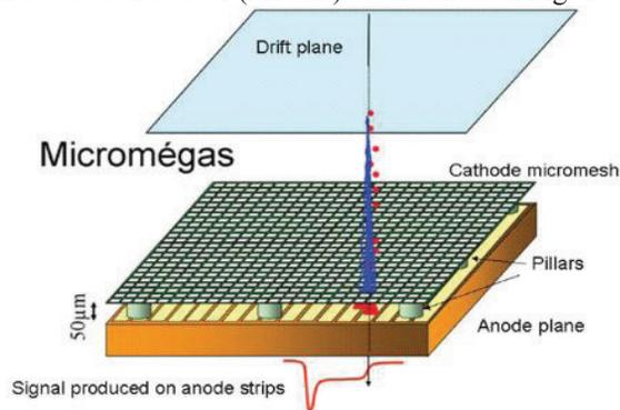
Figure 1: Micromegas scheme.
