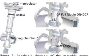
Figure 3: Mechanic drawing of the movable gauge system.
