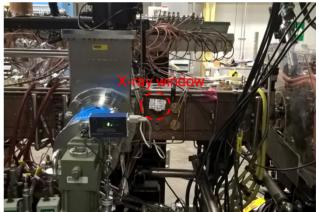
Figure 2: Quartz X-ray window installed in RFQ.
