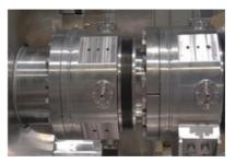
Figure 2: Picture of two of the DBPM's mounted in the Diagnostics Plate.
