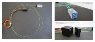
Figure 9: Assembly work of the upgraded new BLM. The photomultiplier tube (PMT) can be separated from the spot area of the beam losses to be connected with the plastic scintillator by the optical fibers.
