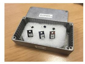
Figure 3: BPW34 Pin diodes and IRF9530 FETs in die cast box.
