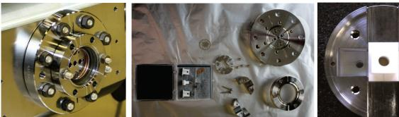
Figure 2: External view of pick-up in BPM body.
