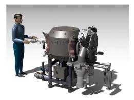
Figure 1: CAD design of AMIT cyclotron.
