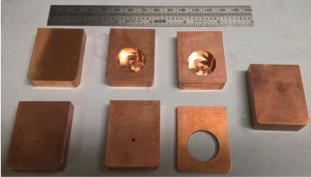
Figure 6: Set of collimators and screens.
