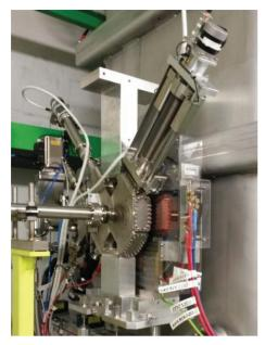
Figure 2: A short DB containing a faraday cup, a scanning slit and a collimating slit installed beside a cryomodule.
