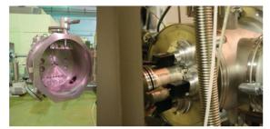
Figure 2: Arrays of scintillators detectors.
