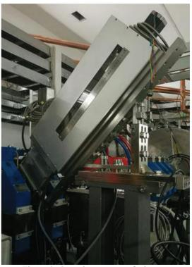
Figure 2: Overview system of wire scanner.
