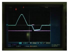
Figure 1a: Pulse kicker current waveform.
