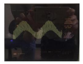
Figure 4: The waveform of the beat frequency signal.
