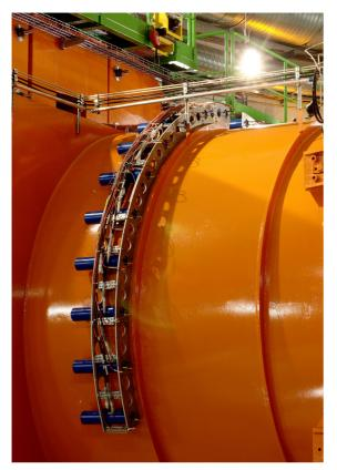
Figure 2: The BHM mounted on the rotating shielding around the beampipe in CMS.
