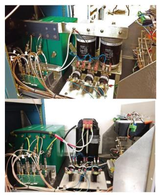
Figure 1: Two interface chassis: One with the resonant capacitors (top) and one with the matching transformer (bottom). The current and voltage transformers are shown in both.
