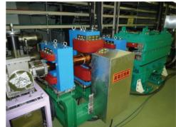
Figure 1: Photo of horizontal IPM system installed at address 76 of J-PARC MR.
