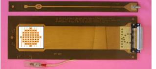
Figure 2: BPM pixel detector for beam profile with 39-pads (bottom) and single-pad (top).
