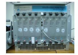
Figure 4: Power supply rack. CPSC is plugged in the center slot and could controller 8 channels of power supplies.
