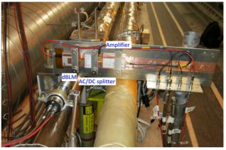
Figure 1: dBLM installation in the LHC IR7.
