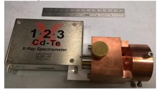
Figure 5: Spectrometer inside copper enclosure.
