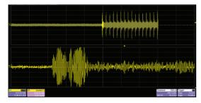
Figure 7: Bunched beam Schottky signals (time domain).
