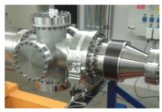
Figure 1: The Fast Current Transformer from Bergoz Instrumentation installed at COSY. The FCT in the ring is equipped with a custom build preamplifier and a current source for calibration. The main parts of the readout and calibration module are installed outside the tunnel.
