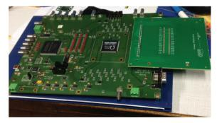
Figure 2: The CITIROC board with the SiPM PCB pluged onto it.
