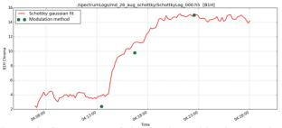
Figure 6: Comparison of chroma derived by the schottky monitor (red line) and chroma as derived with the modulation method (green dots) (Courtesy: M. Wendt, M. Betz).
