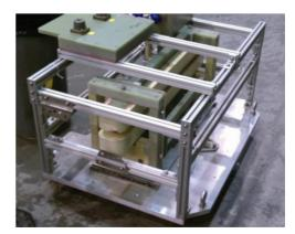
Figure 1b: Original Al frame and baseplate kicker magnet.
