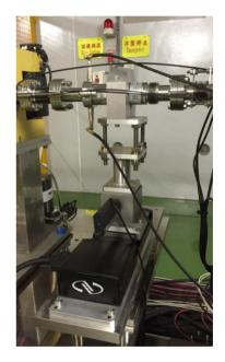
Figure 1: Photograph of the stripline BPM P3 and its mover.
