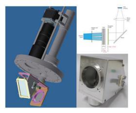
Figure 6: Emittance meter system. (Left) 3D model Schematic of the pepper-pot emittance meter. (Right) scheme of the ion beam imaging system [11].
