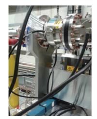
Figure 4: Reentrant BPM (centre) installed on the linac FLASH2 with 180° hybrid couplers.
