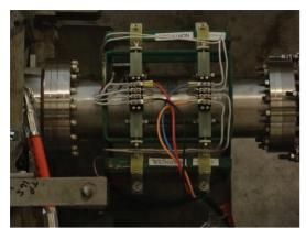
Figure 3b: Post kicker corrector coils installed in the SLAC BSY.
