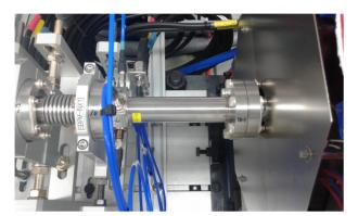
Figure 3: A stripline BPM of the PAL-XFEL linac.
