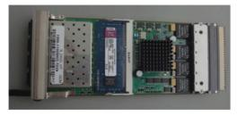
Figure 2: GDX module for FA data grouping and FOFB computation. There are 4 SFP ports provided: two SFP ports for FA data grouping; one SFP for magnet output; one SFP for BPM grouping data output (Gigabit Ethernet).
