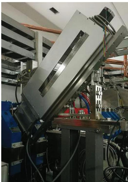
Figure 2: Overview system of wire scanner.
