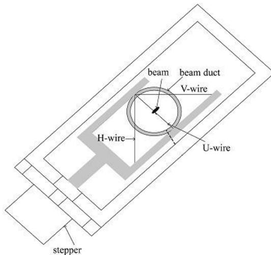
Figure 1: Schematic drawing of the wire scanner.
