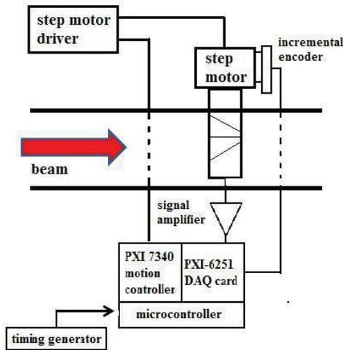
Figure 3: A schematic diagram of wire scanner.
