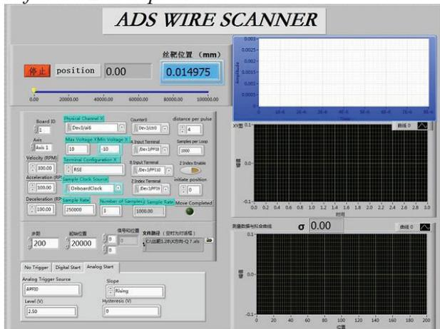
Figure 4: Graphic interface of the LabView based application for wire scanner.
