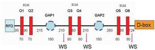
Figure 5: The layout of MEBT-1 for CADS injector-I.
