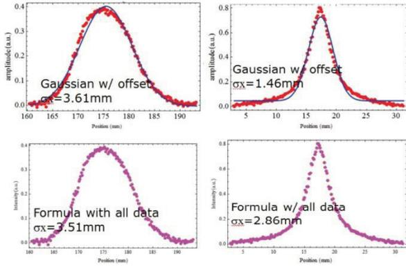
Figure 6: Fitting results for wide-plump and narrow-pointed signal with two different fitting methods.
