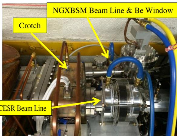
Figure 3: NGXBSM vacuum components.
