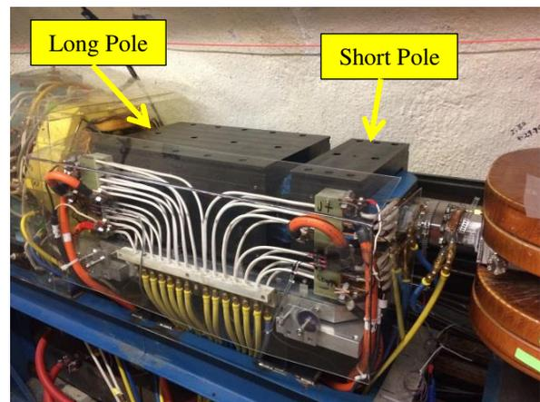
Figure 4: NGXBSM source magnet.
