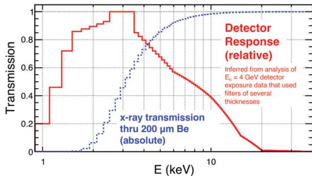
Figure 6: Detector response and Be window transmission.
