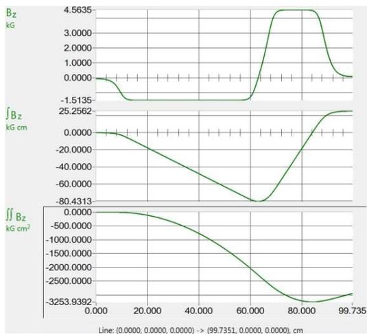
Figure 5: Magnetic field map of NGBSM magnet.
