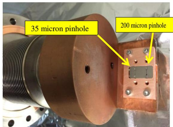
Figure 11: NGXBSM pinhole stage.
