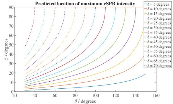
Figure 4: Predicted locations of peak cSPR intensity according to Eq. 3 for a particle beam with  $\gamma=39000$  and  $n = m = 1$ .
