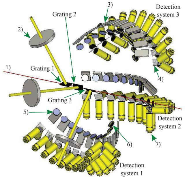
Figure 2: The proposed layout of a single-shot longitudinal profile monitor. The components are: 1) beam path, 2) vacuum feedthroughs, 3) mirrors, 4) polarizers, 5) vacuum windows, 6) filters and 7) concentrators and detectors. Grating 1 illuminates detection system 1. Components are to scale. Schematic drawn using CST Microwave Studio [7].
