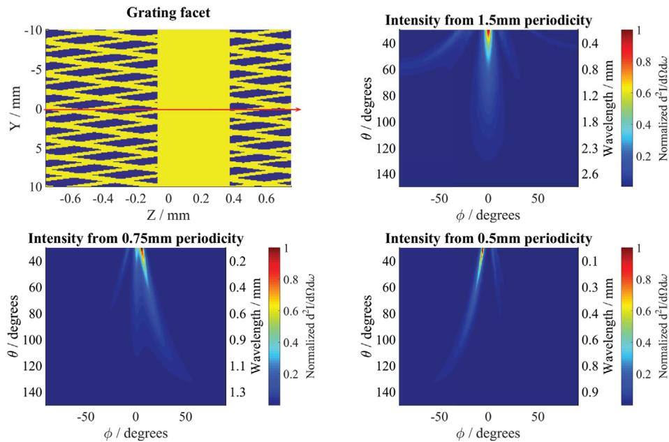
Figure 5: A facet which combines three gratings of different periodicities into a single grating. Yellow indicates conductor, blue indicates vacuum and the beam propagation direction is shown by the red arrow. The calculated intensity distributions associated with each periodicity predict that the radiation should be spatially and spectrally separated.
