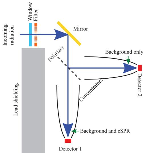
Figure 1: Two detector system to enable background subtraction on a shot-by-shot basis. By subtracting the signal from detector 2 from the signal from detector 1 it is possible to extract the SPR signal without backgrounds (assuming that it is perfectly polarized).
