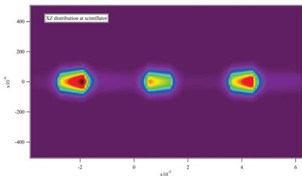
Figure 5: 2D distribution at the scintillator location. XZ grid: 151 x 151 over 10 x 1 mm. Initial photon distribution: 100 photons from 50 up to 200 keV. Fe thickness: 20 mm.
