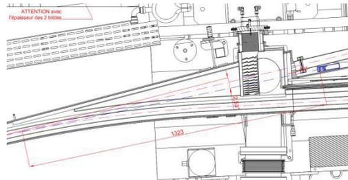
(a) Chamber drawing. Scintillator in blue.
