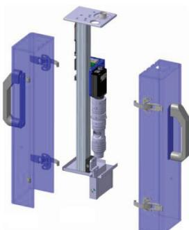
Figure 7: 3D view of the detector and its mechanics.
