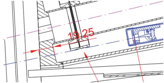
Figure 4: Dipole chamber exit. Scintillator in blue.
