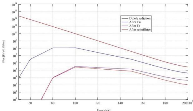
Figure 6: SR spectrum at various stages of the process. Integration over the 10 x 1 mm transverse window at the scintillator location. Fe thickness: 20 mm.
