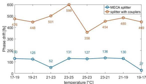
Figure 8: Setup II. Drift per 2°C steps (between mean values of each step).
