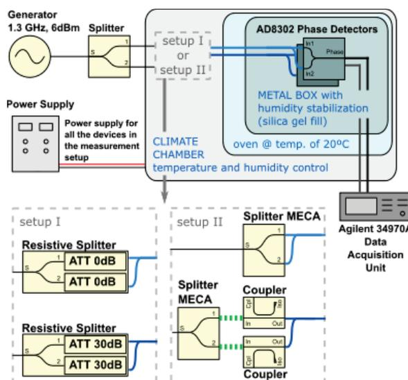
Figure 2: Measurement setup schematic.
