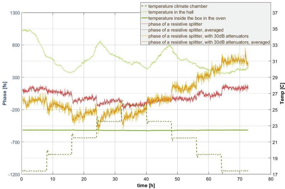
Figure 3: Setup I. Phase difference measured at 1.3 GHz between the outputs, and environmental temperature vs. time.
