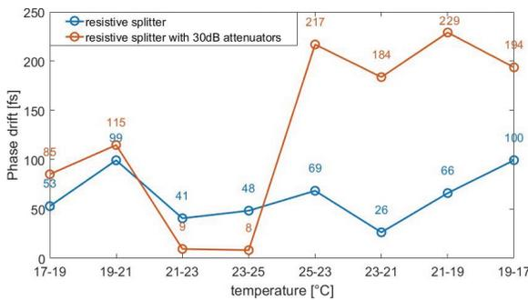
Figure 5: Setup I. Drift per 2°C steps (between mean values of each step).
