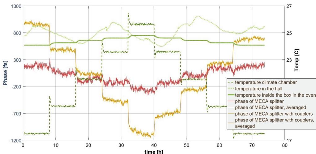
Figure 6: Setup II. Phase difference measured at 1.3 GHz between the outputs, and environmental temperature vs. time.
