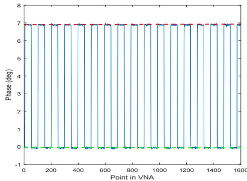
Figure 3: Phase delay between the long and short cables for a 10 Hz switching frequency.
