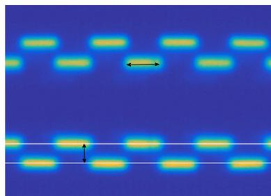
Figure 2: Output image of the streak camera after performing the delay of the 250MHz signal with the RF switches.
