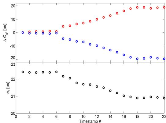
Figure 5: Centroid position (top) and bunch length (bottom) evolution during an RF cavity recovery. The RF voltage goes from 2.3 MV to 2.6 MV in about 5 min, and each timestamp corresponds to approximately 14 sec.
