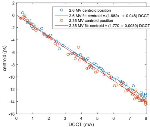
Figure 8: Centroid displacement during an injection in single bunch mode for  $V_0=2.5$  MV and  $V_0=2.35$  MV.
