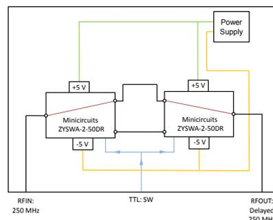
Figure 1: Schematic illustration of the crate used in order to introduce a delay in the 250MHz signal using the PIN diodes switching with a frequency set by the TTL signal and two cables with a certain different length.
