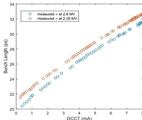
Figure 7: Change of the bunch length during the injection in single bunch mode. The profiles in Fig. 6 are fitted to a simple Gaussian curve.
