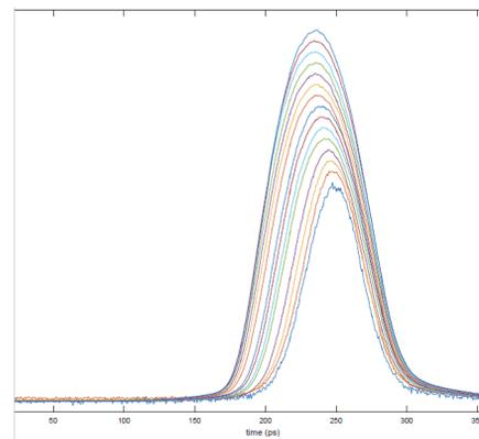
Figure 6: Mountain range plot while increasing the bunch intensity from 0.5 mA (lower trace) to 8 mA (top).
