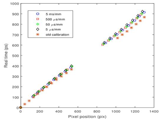
Figure 4: Multilinear calibration for different sweep speeds and using the old calibration from the Michelson interferometry [2]. For the sweep speeds from 5ms/mm to 5 $\mu\text{s}/\text{mm}$  the multilinear calibration is almost identical.
