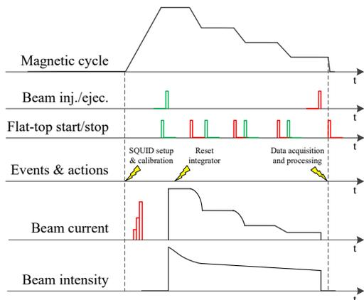
Figure 4: Actions and events during the AD cycle acquisition.
