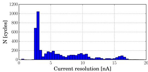
Figure 6: Distribution of the current resolution for 4685 acquired cycles.
