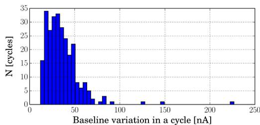
Figure 7: Distribution of the baseline drift for 271 acquired cycles where no beam was injected.
