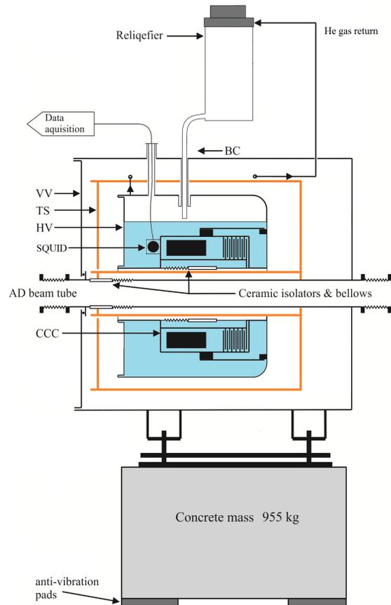
Figure 3: CCC cryostat schematic.
