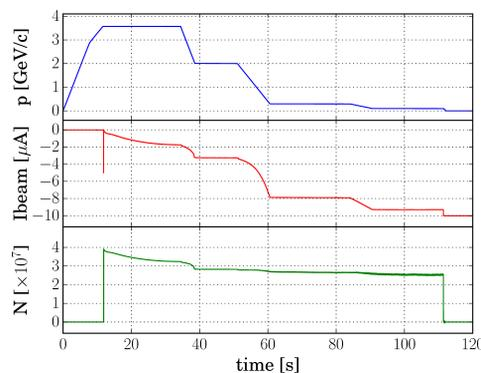
Figure 5: Measurement of the AD cycle beam current in red (middle) and intensity in green (bottom), with the particle momentum shown in blue (top).
