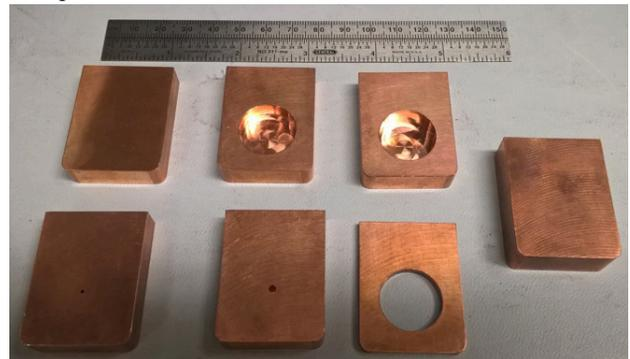
Figure 6: Set of collimators and screens.
