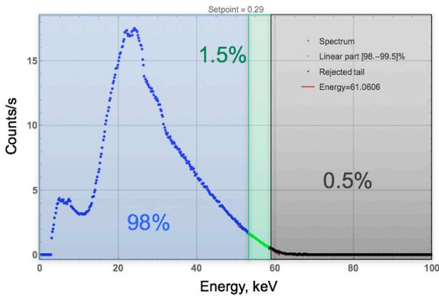
Figure 3: Typical spectrum measured by unshielded spectrometer.
