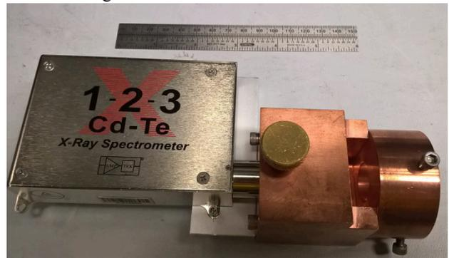
Figure 5: Spectrometer inside copper enclosure.
