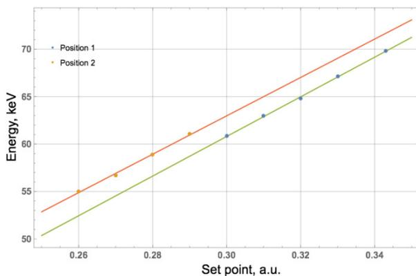
Figure 4: Measured X-ray energy vs RFQ set point taken in two different positions: orange – facing directly the window, green – moved 30 cm away and slightly misaligned.
