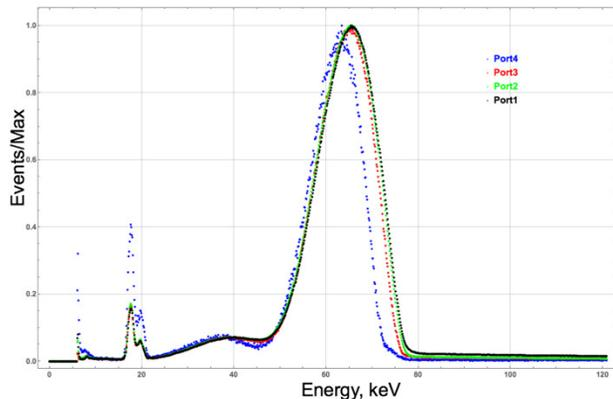
Figure 7: X-ray spectra at different ports, normalized over peak maximum.
