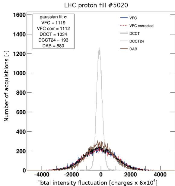
Figure 9: Noise performance of different intensity measurement systems.
