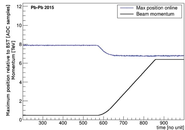
Figure 4: Evolution of the phase between the bunch apex and the BST clock during the acceleration of lead ions in the LHC. The blue trace shows the measured phase while the black trace shows the beam energy.
