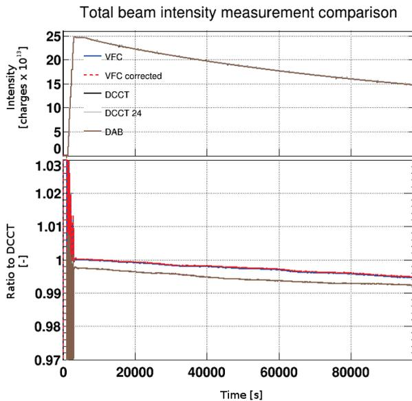
Figure 8: Comparison of the digital intensity measurement method with the DCCT and analogue measurements.
