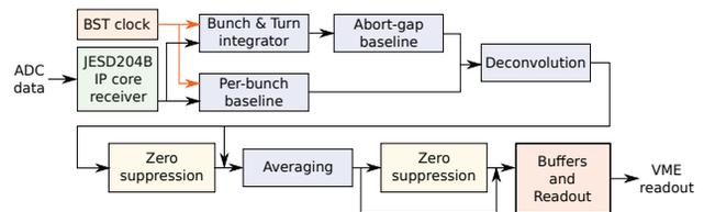
Figure 3: The FPGA data processing flow.
