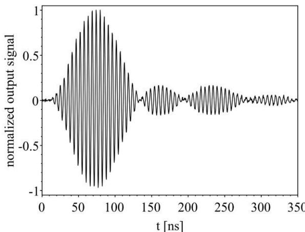
Figure 6: Normalized Turbo-ICT output signal measured on an oscilloscope.
