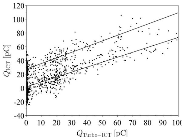
Figure 7: For the capillary-discharge based LPA, charge measured by the ICT versus charge measured by the Turbo-ICT. The data splits into two parallel bands. The lines are linear fits to these bands.
