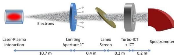
Figure 3: Schematic of the measurement setup
