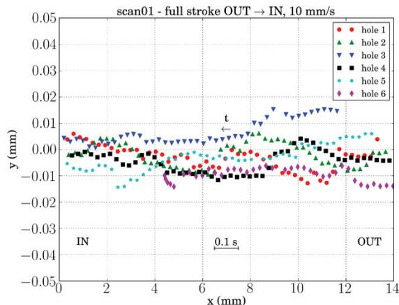
Figure 7: Tracking of the hole positions in the x-y (camera) plane. The blade speed was 10 mm/s, and the movement was from the fully OUT to the fully IN positions.
