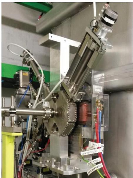
Figure 2: A short DB containing a faraday cup, a scanning slit and a collimating slit installed beside a cryomodule.
