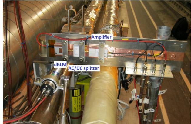
Figure 1: dBLM installation in the LHC IR7.
