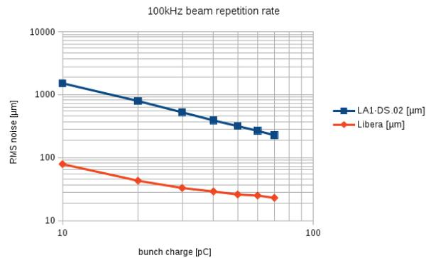
Figure 7: Measured beam position noise at 100 kHz bunch repetition rate.
