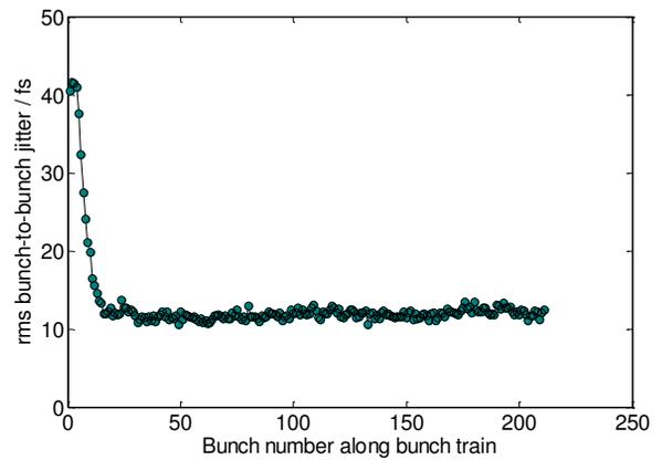
Figure 9: The BAM and BBF application performance at 3DBC2 BAM at FLASH.
