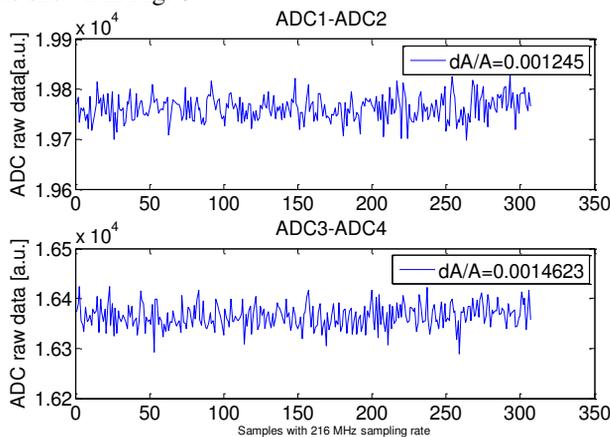
Figure 8: ADC stability measurements for the BAM signals detection of 3DBC2 detector.
