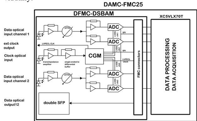
Figure 4: The block diagram of MTCA.4 based OFR electronics.
