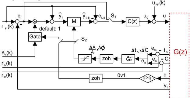
Figure 3: Functional block diagram for the intra-train beam based feedback.
