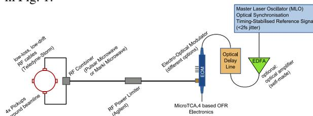
Figure 1: The block diagram of BAM detector.
