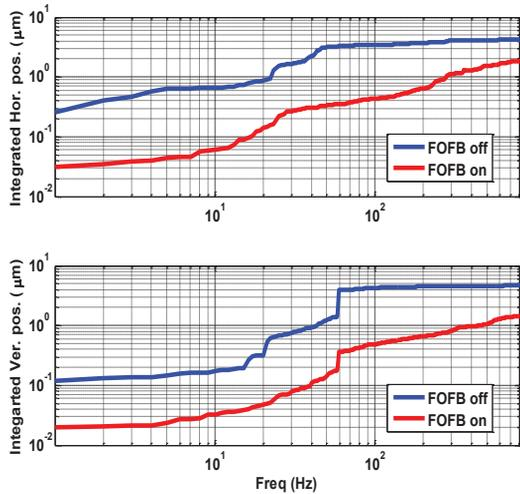
(a) Integrated BPM position displacement
