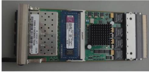
Figure 2: GDX module for FA data grouping and FOFB computation. There are 4 SFP ports provided: two SFP ports for FA data grouping; one SFP for magnet output; one SFP for BPM grouping data output (Gigabit Ethernet).
