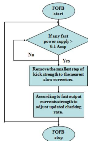
Figure 9: FOFB with slow corrector compensation to avoid fast corrector saturation.
