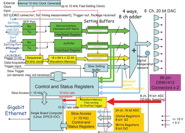
Figure 5: Functional block diagram of the corrector power supply controller module. The EPICS channel access is via a dedicated embedded IOC. The fast setting from feedback engines would sum with the EPICS CA slow setting.
