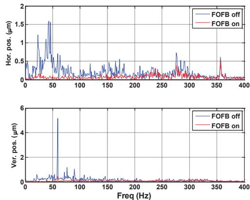
Figure 6: Beam Spectrum (no booster power supply ramping).
