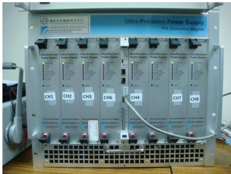
Figure 4: Power supply rack. CPSC is plugged in the center slot and could controller 8 channels of power supplies.
