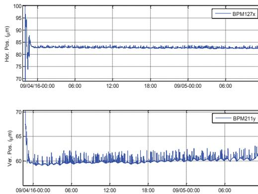
Figure 10: Horizontal and vertical orbit with FOFB and RF feedback during 36 hours of operations. There are some spikes due to injection around every 5 minutes.
