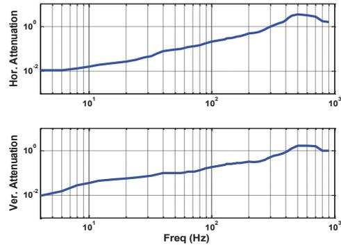
Figure 8: The measured bandwidth of FOFB. Horizontal is around 250Hz and vertical around 300 Hz.
