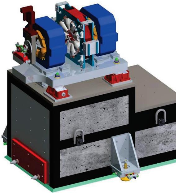
Figure 5: ID BPM concrete support system.
