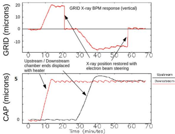
Figure 2: Impact of mechanical motion for ID BPMs.
