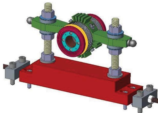
Figure 4: Bellows isolated BPM.
