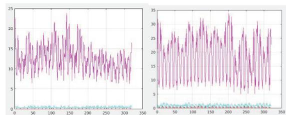
Figure 4: Orbit distortion rms due to random quadrupole displacements (purple) and rms of orbits corrected using the full (red) or reduced set (blue) of BPMs and correctors
