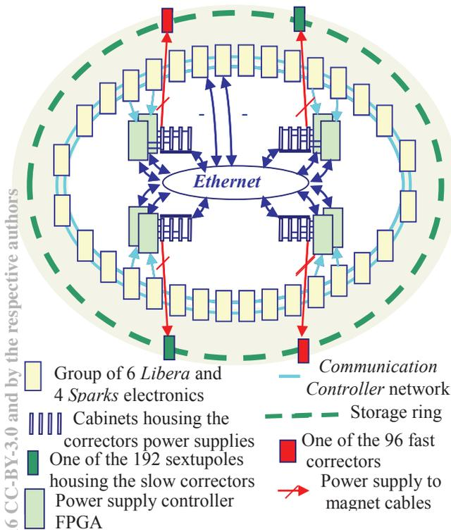
Figure 2: Layout of the EBS orbit correction system.
