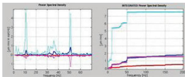
Figure 6: Spectrum of the orbit distortion (left plot). Integrated spectrum of the orbit distortion (right plot). Light blue/horizontal without feedback, dark blue/horizontal with feedback, purple/vertical without feedback, red vertical with feedback
