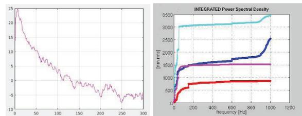
Figure 3: Left plot: fast PID correction effect versus frequency in dB Right plot: integrated spectrum of the orbit distortion; Light blue/horizontal without feedback, dark blue/horizontal with feedback, purple/vertical without feedback, red vertical with feedback.
