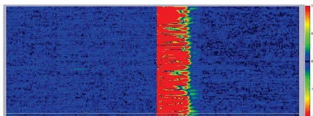
Figure 7: Display of the stability of the orbit stability with the hybrid slow/fast correction scheme (left part) and the normal correction scheme (right part).
