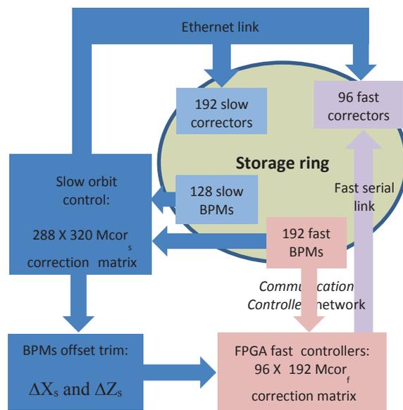
Figure 5: Layout of the control of the orbit correction system used for the test.
