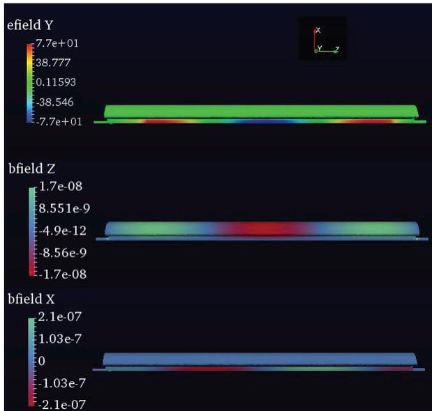
Figure 5: RF fields distribution of the 3<sup>rd</sup> mode. Top: E<sub>y</sub>; Middle: B<sub>z</sub>; Bottom B<sub>x</sub>.
