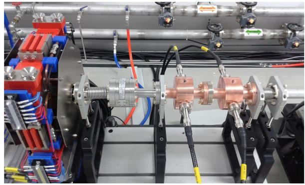
Figure 7: A Turbo-ICT and beam arrival-time monitors of the PAL-XFEL linac.
