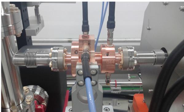
Figure 4: A cavity BPM of the PAL-XFEL undulator section.
