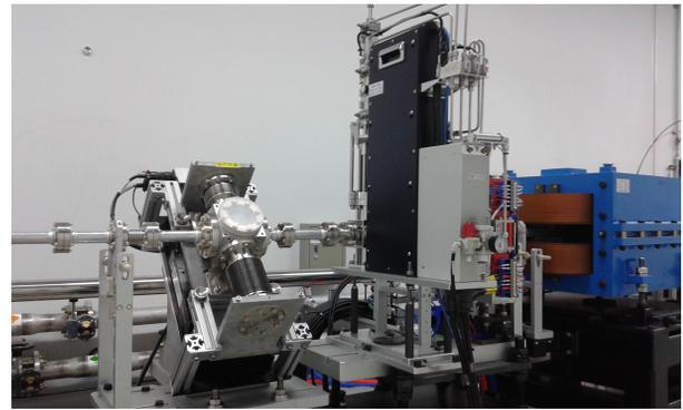
Figure 5: A wire scanner (left) and a screen monitor (right) to measure the transverse beam profile.
