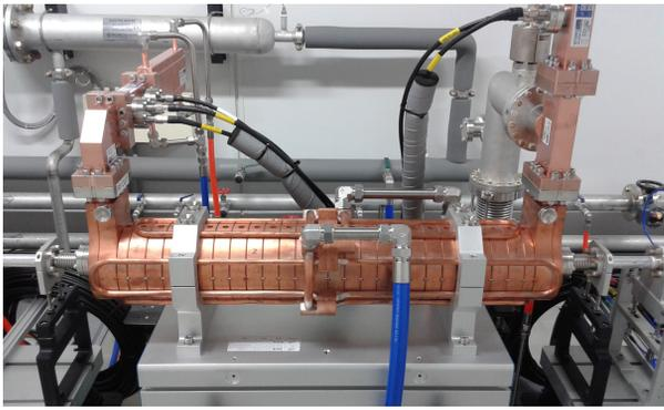
Figure 6: A deflecting cavity for the measurement of the longitudinal bunch length.
