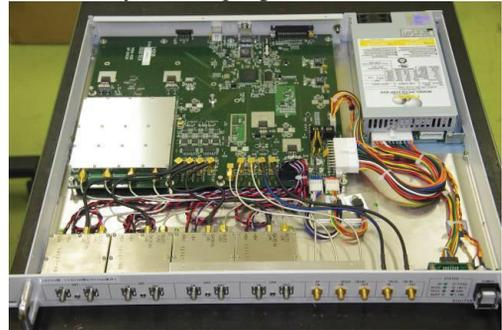
Figure 4: Photo of the gated turn-by-turn detector.
