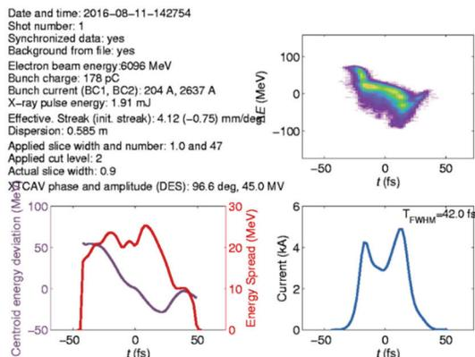
Figure 6: Streaked image (top right), longitudinal charge profile (bottom right) and reconstructed photon profile (bottom left) during non-SLED operation.
