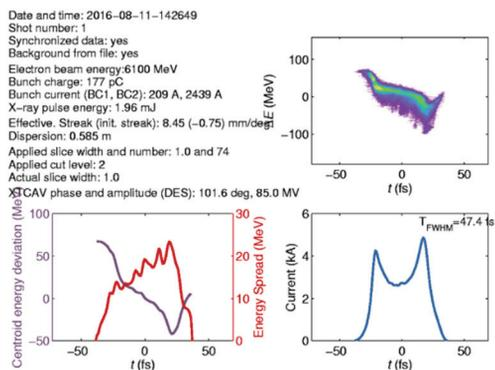
Figure 7: Streaked image (top right), longitudinal charge profile (bottom right) and reconstructed photon profile (bottom left) during SLED operation.
