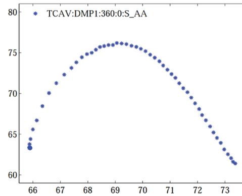
Figure 4: Temperature sensitivity of the SLED cavity is shown when the output power [MW] is plotted versus temperature [deg. F].
