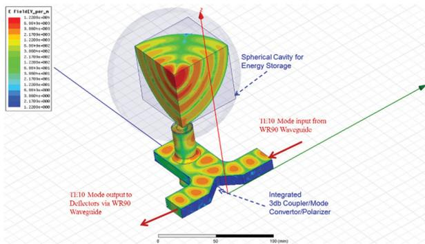
Figure 3: The incoming TE01 waveguide mode converts to two TE11 modes in the circular guide which couples to the two circularly polarized spherical modes in the cavity.
