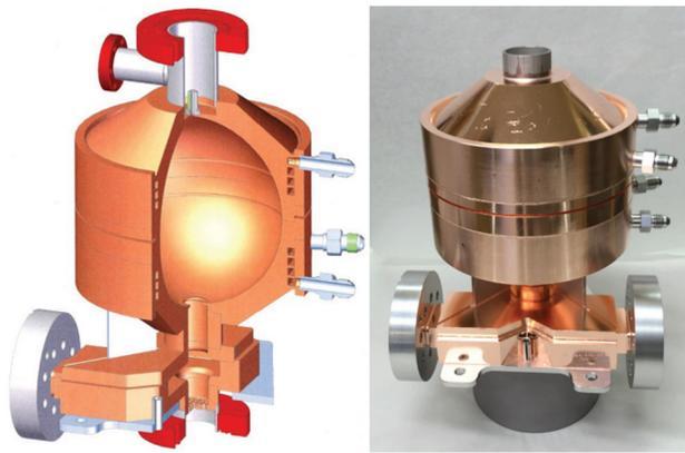
Figure 2: Cut-away view of the X-band SLED cavity together with a photo of the brazed cavity and coupler assembly.
