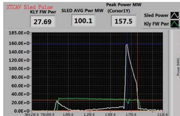
Figure 5: SLED RF output pulse from the SLED cavity (white) peaks rapidly when the phase is reversed and gives 4 times the average power in the last 200 ns compared to the 1 us pulse from the klystron (green).
