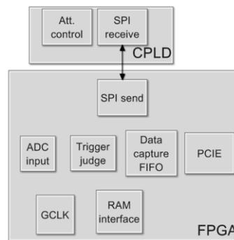
Figure 6: Firmware structure.
