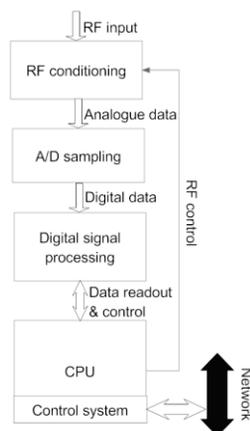
Figure 1: DBPM processor architecture.
