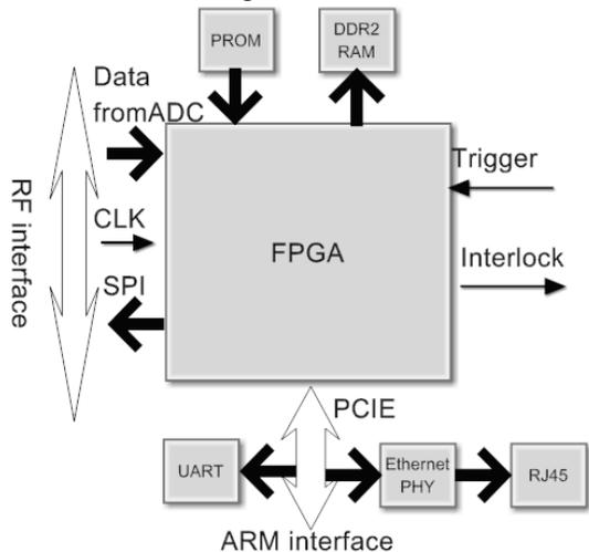
Figure 4: Mother board hardware block diagram.
