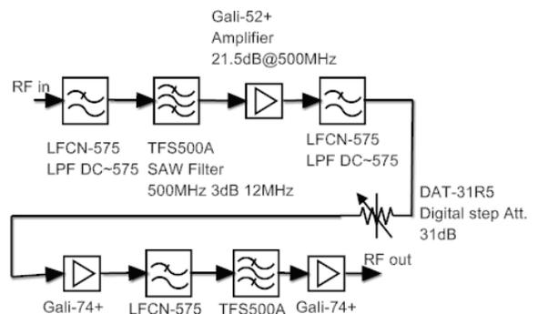
Figure 3: RF conditioning flow.
