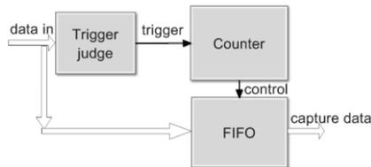
Figure 7: Self-trigger module.
