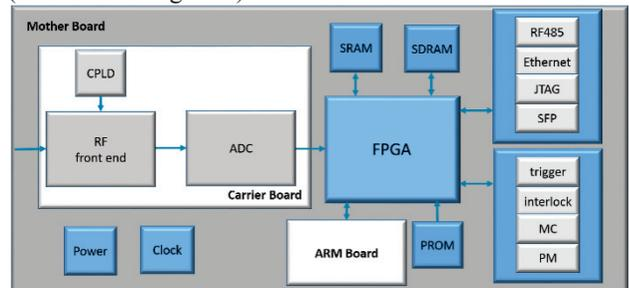
Figure 2: Hardware diagram.
