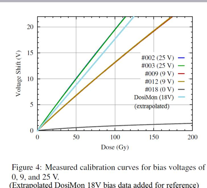
Figure 4: Measured calibration curves for bias voltages of 0, 9, and 25 V.
