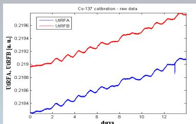
RadFet threshold voltage raw data (both channels)
