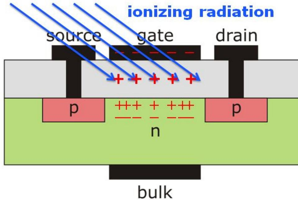
ionizing radiation → stationary charges in insulation layer
