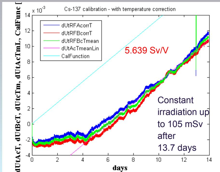
Temperature-corrected threshold voltage vs time
