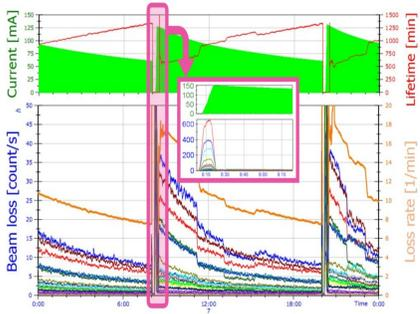
Machine operation status. The beam loss signal during injection process is expanded in the pink box.
