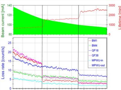
Beam loss for three different emittances without IDs at the beam energy of 1.2 GeV.
