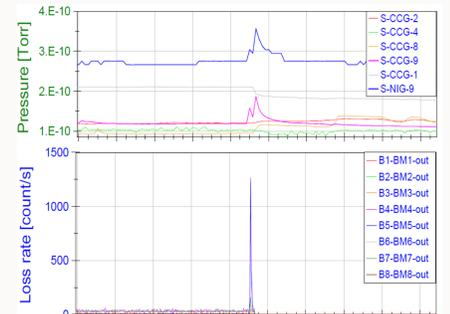
Beam loss and vacuum pressure during the beam dump.
