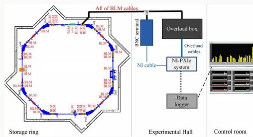
The sketch map of BLM system. The detectors are two PIN-diodes from Bergoz. The real-time loss rate is recorded at each point of the storage ring and updated every second by NI-PXIe system.
