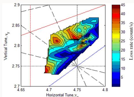
Beam loss rate versus tune scanning for the SPS storage ring with the emittance of 61 nm-rad.
