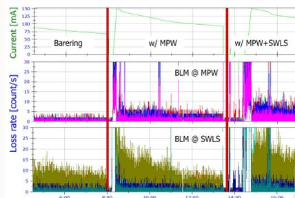
Beam loss for three modes of machine operation (Bare ring w/o IDs, 2.2 T MPW, and 4.0 T SWLS + 2.2 T MPW).
