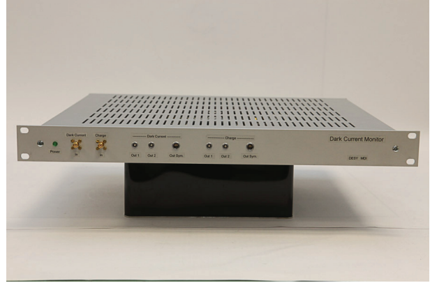
Figure 4: Photo of the DaMon electronics. From left: power control LED, dark current input, beam charge input, 3 dark current outputs (2 times single ended and 1 differential), 3 beam charge outputs.
