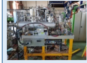
ARIBE: characterization of Ar 8+ beam at 30 keV and commissioning of beam focusing prototype
