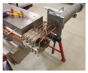
water and current supply of the single coil windings
