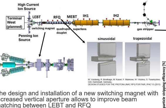
Main step to higher uranium intensity is related to pulsed gas stripper operation with Hydrogen
