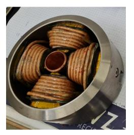
*inner yoke with magnet coils*
