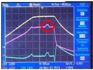
RF amplitude (yellow) and RF power signal (magenta): additional power needed during beam pulse
