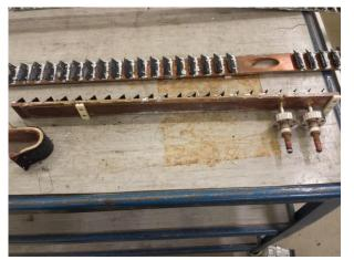
defect baffle plates with corrosion
