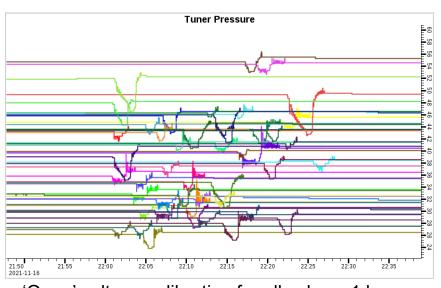
'Open' voltage calibration for all valves: 1 hour
