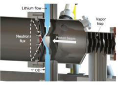
FIGURE 3. LiLiT target, for details see [5]. The sample to be irradiated by the neutrons can be placed at about 1 cm from the target (the red line) and is exposed there to neutron flux of about  $2 \times 10^{10} \text{ n/s/cm}^2\text{mA}$
