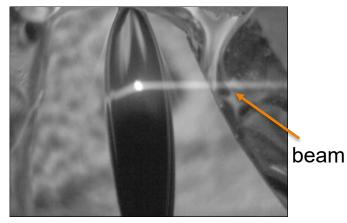
Film being irradiated by proton beam
