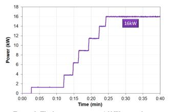
Figure 6: The beam power up to 16 kW proton beam.
