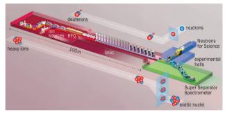
Figure 2: A schematic view over the SPIRAL2 installation, the two injectors on the right hand side.
