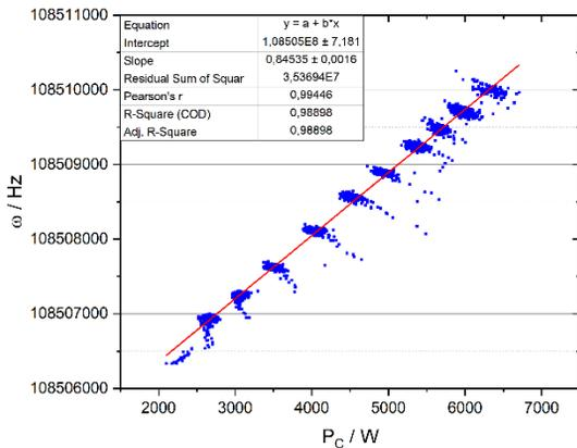
Figure 5: Calculated thermal detuning of the RFQ prototype.
