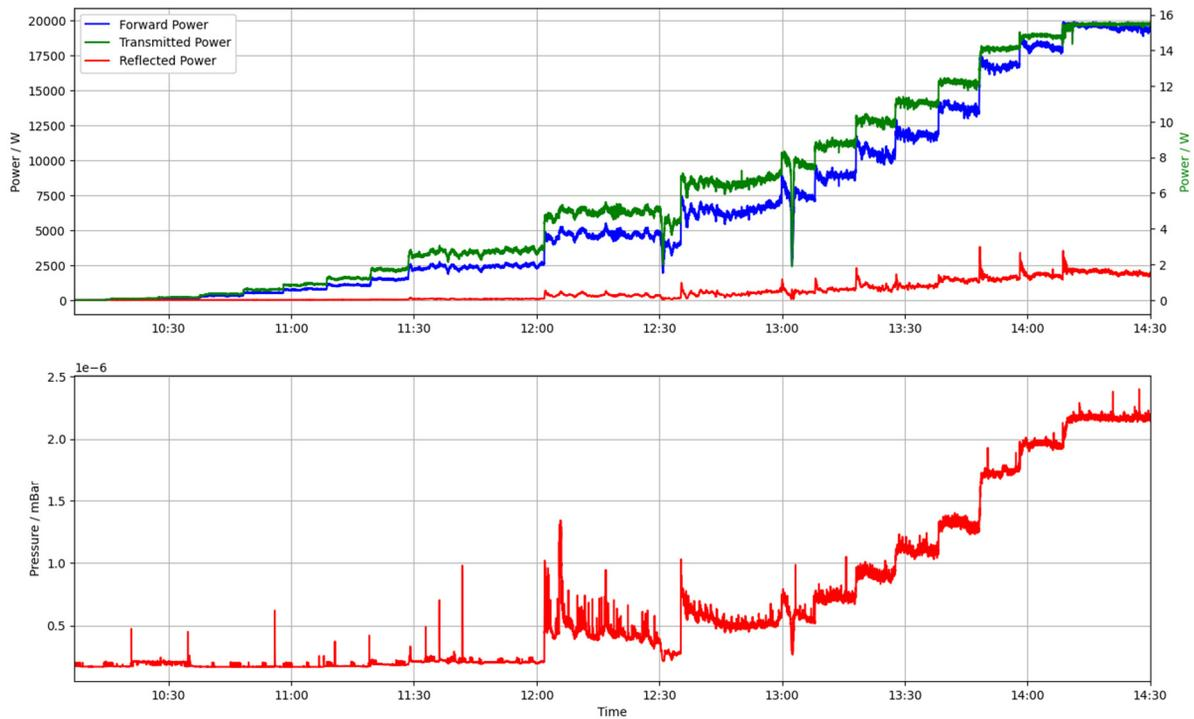
Figure 3: Conditioning process from 0 W up to 20 kW median forward power.
