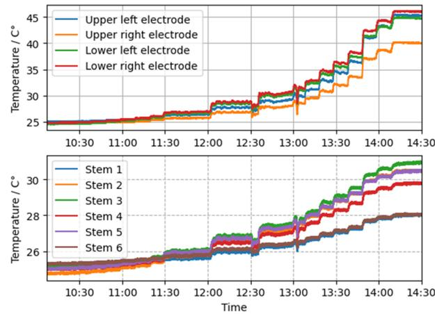
Figure 4: Measured cooling water temperatures for selected points, corresponding to the RF conditioning depicted in Figure 3.
