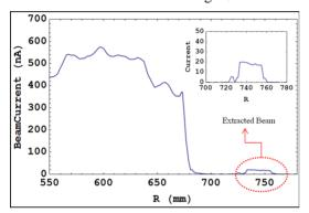
Figure 13: Beam current vs. radius for N<sup>2+</sup>, 4.5 MeV/u beam ( $f_{rf} = 14$  MHz, in 2<sup>nd</sup> harmonic mode of operation); First deflector entry was at 668.0 mm.
