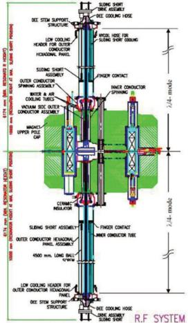
Figure 6: Half-wave coaxial RF cavity of SCC.
