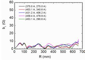
Figure 12: 1st harmonic amplitude at different excitations of main coils.
