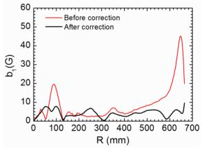
Figure 11: 1<sup>st</sup> harmonic field before and after correction of cryostat position.
