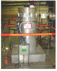
Figure 8: Tetrode based final RF Amplifier.
