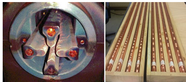
Figure 4: Installed HSI RFQ electrodes after 10 years' operation (left); newly fabricated electrodes just before assembly (right).
