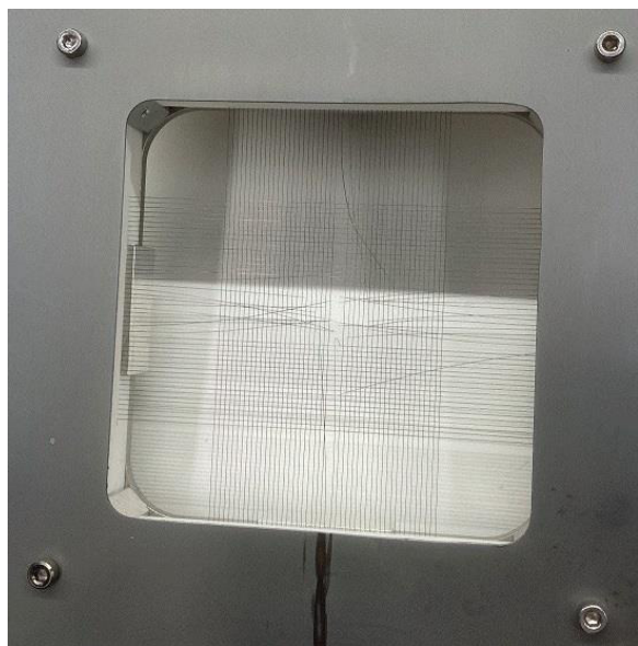
Figure 6: Damaged SEM profile grid.
