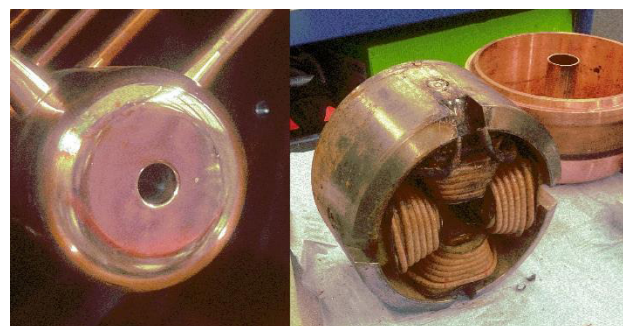
Figure 2: Drift tube of Alvarez section, as installed (left); opened drift tube with defective quadrupole lens (right).
