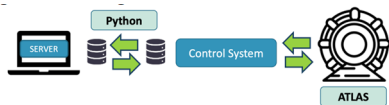
Figure 4: Scheme representing the communication with the Control System from an existing server through the new python package.
