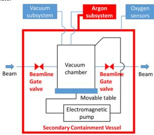
Figure 2: FRIB liquid lithium charge stripper system. The liquid lithium loop is completely enclosed by a secondary containment vessel as a safety control. Noted by red are safety controls.
