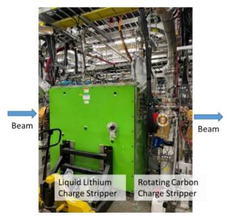
Figure 10: Photograph showing the LLCS and the carbon charge stripper connected in series in FS1 of the FRIB linac. The LLCS is located upstream of the carbon stripper.
