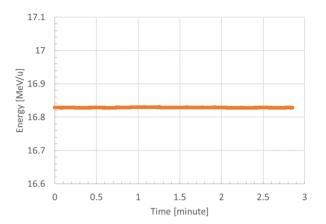
Figure 7:  ${}^{36}$ Ar beam energy after the lithium stripper during the high-intensity irradiation test (peak intensity 12 particle  $\mu$ A, peak beam power 7400 W (average 400 W, duty cycle 5.4%), peak power loss 50 W (volumetric power deposition 6 MW/cm<sup>3</sup>).
