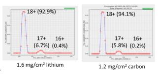
Figure 6: Charge state distributions of 20 MeV/u argon beam after the LLCS and carbon foil stripper. Thickness was  $1.6 \text{ mg/cm}^2$  and  $1.2 \text{ mg/cm}^2$  for the lithium and the carbon, respectively.
