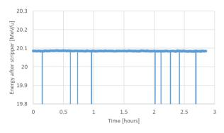
Figure 9: <sup>48</sup>Ca beam energy after the lithium stripper. At downward spikes the beam was tripped.
