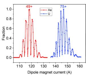
Figure 5: Xenon (red) and uranium (blue) charge state distributions after the liquid lithium stripper. The thickness is  $1.05 \text{ mg/cm}^2$  for the xenon beam and  $1.40 \text{ mg/cm}^2$  for the uranium beam.
