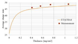
(a) Average charge states of xenon beam stripped by lithium.
