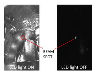
Figure 8: Beam spot on the LLCS during the high-intensity irradiation test. The LED light was turned off on the right photo to take a clear beam spot.
