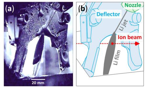
Figure 3: Liquid lithium charge stripper formed in a vacuum chamber which is part of the FRIB linac beamline. (a) Photograph of the lithium film and (b) sketch of what's seen in the photograph. A round jet of liquid lithium being issued from a nozzle impinges on a flat surface ("deflector"). The jet is then deflected forming a stable film that intercepts beams. The film is stable enough to have a mirror surface that reflects the surrounding components in the vacuum chamber or its inner wall.
