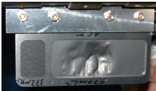
Figure 7: Target frame of the transfer channel foil stripper with two foils mounted in a slot of the foil carousel. The large foil shows deformation caused by the energy deposition of the beam.
