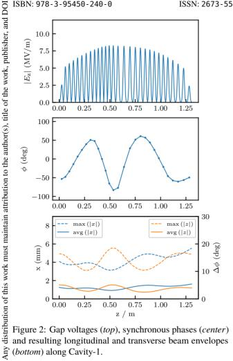
Figure 2: Gap voltages (top), synchronous phases (center) and resulting longitudinal and transverse beam envelopes (bottom) along Cavity-1.
