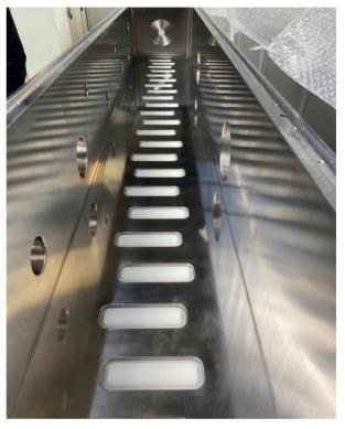
Figure 3: RFQ stainless steel tank with cut outs for the stems.
