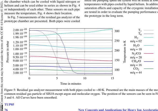
Figure 5: Residual gas analyzer measurement with both pipes cooled to ≈80 K. Presented are the main masses of the most common residual gas particle of SIS18 except argon and molecular oxygen. The position of the sensors can be seen in Fig. 3 and 4. All Curves have been smoothed.
