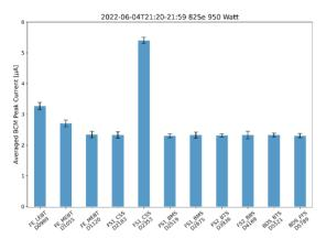
Figure 7: The <sup>82</sup>Se beam current averaged over the 60 sec along the linac. The error bar shows the standard deviation due to the noise in the signal. The D-numbers near the horizontal axis show the location of the BCMs along the linac in decimeters. The first BCM is located upstream of the RFQ. The last BCM is located upstream of the target.
