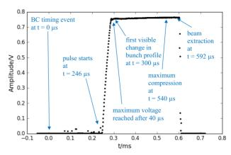
Figure 7: Bunch compressor voltage amplitude, scale 1:40,000 (obtained by a sine fit algorithm on the measured gap voltage signal; the smaller outliers before the pulse are numerical artefacts of the sine fit).
