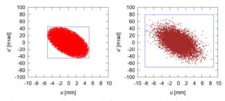
Figure 3: 4D Waterbag (left) and Gaussian (right) transverse input distributions (*u* represents the *x* or *y* direction).
