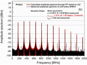
Figure 9: Comparisons between the calculated by Eq. (7) and the measured output voltage of cold button BPM19 in TD (a) and FD (b) during proton beam commissioning. ingly, the amplitude spectra in FD is coincided with together, as shown in Fig. 9(b). The induced imaging bunch shape and the amplitude of signal could have a good agreement with the measured results regardless of whether the signal is
