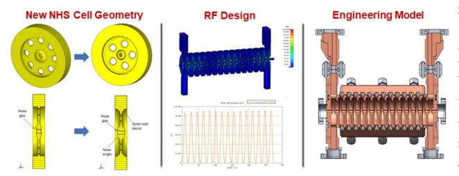
Figure 6: New cell geometry, rf design and engineering model for the latest NHS design developed by Radiabeam.
