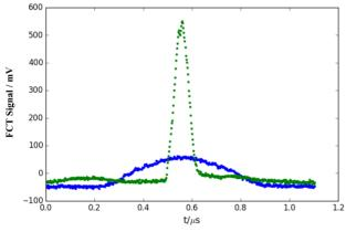
Figure 6: Comparison of bunch profiles before (blue) and at maximum compression (green).
