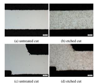
Figure 5: Prepared cross sections of printed KF40 pipe wall material (bright areas = steel). The top images show a cross-section of the pipe wall, the bottom images show the region around the KF 40 flange. Courtesy of GSI Darmstadt, pLinac project.
