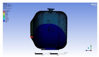
Figure 10: 2nd Mode – Free Cover Fluctuation.
