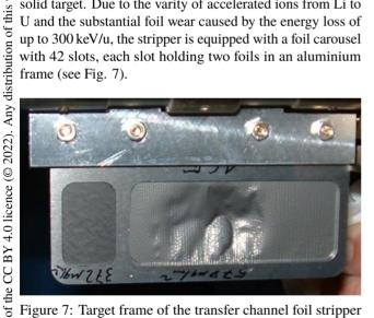
Figure 7: Target frame of the transfer channel foil stripper with two foils mounted in a slot of the foil carousel. The large foil shows deformation caused by the energy deposition of the beam.
