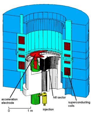
Figure 3: Schematic 3D-model of the AGOR cyclotron interior.
