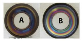
Figure 1: The image of the 1st (A) and 12th (B) Ti electrode removed from tube 1 in unit 19 after ~40 years of operation. Left image (A) is the discoloured electrode surface facing the top of accelerator and (B) is the surface of the 12th tube electrode facing the bottom of accelerator.
