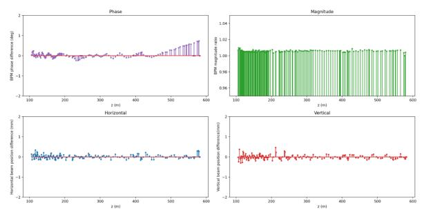
Figure 6: BPM readings during the operation. Plots show the difference between the readout and reference setting of the linac for the bunch phase (top-left), horizontal and vertical (bottom) beam positions. Plot (top-right) shows the BPM signal magnitude normalized to the reference signal strengths.
