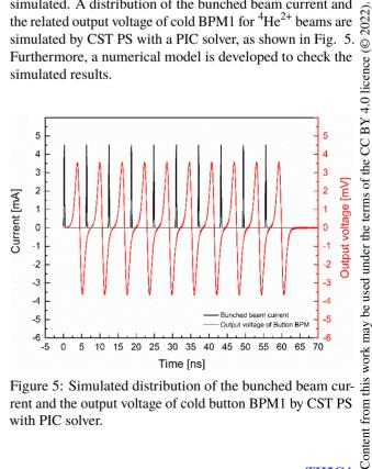
Figure 5: Simulated distribution of the bunched beam current and the output voltage of cold button BPM1 by CST PS with PIC solver.
