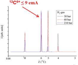
Figure 7: Stripper spectrum optimized for C<sup>6+</sup>. [6]
