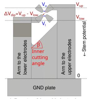
Figure 4: Front view of the model, showing the stem for one cell.  $V_{up}$  and  $V_{low}$  showing the potentials of the long and short arm in reference to the ground plate,  $\Delta V_{dip}$  is the resulting dipole voltage.  $V_u$  and  $V_l$  are the calculated voltages used for the dipole factor calculation.
