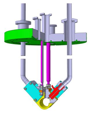
Figure 5: Sketch of the latest stripper setup accomodating two fast valves for gaseous media. One valve is indicated in red. Gas supply is from top via the tubes. The interaction zone is within the yellow tube at the bottom.
