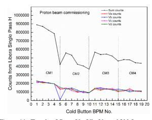
Figure 11: Trends of Sum, Va, Vb, Vc and Vd from cold button BPM1 to BPM19. These data are from the BPM electronics of Libera Single Pass H. The recording time is from 22:08 to 22:49 on Feb. 3, 2021.
