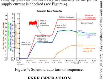
Figure 4: Solenoid auto turn on sequence.
