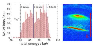
Figure 3: Left: energy distribution of decelerated ions behind the RFQ (simulation). The image on the right-hand side shows the energy spectrum recorded on the RFQ single-shot energy analyzer.
