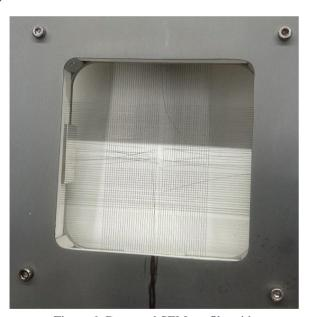
Figure 6: Damaged SEM profile grid.
