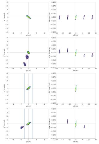
Figure 7: Y-Y' (left) and longitudinal (right) beam snapshots simulated by TRACK: before the chopper, after the chopper, before the beam dump, and after the beam dump (vertical lines represent aperture size).
