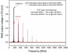
Figure 12: Comparison between the calculated signal in FD of cold button BPM1 and BPM19 during <sup>4</sup>He<sup>2+</sup> beam commissioning.
