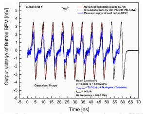
Figure 7: Comparisons between the simulation by CST PS with PIC solver, the numerical calculation by Eq. (6) and the measured output voltage of cold button BPM1.
