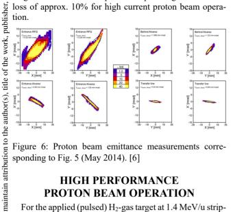
Figure 6: Proton beam emittance measurements corresponding to Fig. 5 (May 2014). [6]
