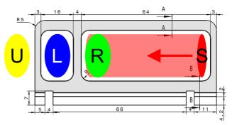
Figure 8: Illustration of the four operating modes of the transfer channel foil stripper. Coloured ellipses indicate the beam spot positions wrt the foil frame (grey) for the different operating modes. Blue spot (L) and Green spot (R): Static stripping via the left, small foil and the right, large foil, respectively. Yellow spot, U: Unstripped mode. Red spot, S: Sweeper mode, the beam spot position at the start of the beam pulse is indicated, while the light red area depicts the foil painting.
