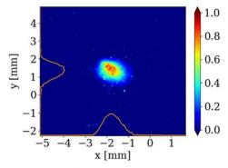
Figure 9: The 1 kW <sup>82</sup>Se beam image on the beryllium target.
