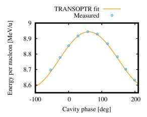
Figure 4: Energy vs cavity phase plot for one cavity, showing resulting fit between measured behaviour and the model.
