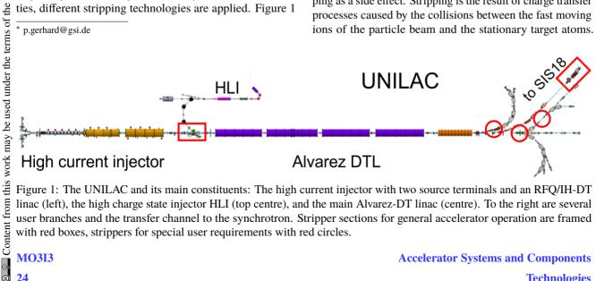
Figure 1: The UNILAC and its main constituents: The high current injector with two source terminals and an RFQ/IH-DT linac (left), the high charge state injector HLI (top centre), and the main Alvarez-DT linac (centre). To the right are several user branches and the transfer channel to the synchrotron. Stripper sections for general accelerator operation are framed with red boxes, strippers for special user requirements with red circles.
