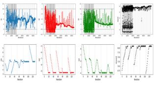
Figure 17: Results obtained for a baseline RL model using DDPG and the TRACK Code. The model optimized the beam size by varying 3 electrostatic quadrupoles. (Top) The results of the training. (Bottom) The results for 5 different predictions starting from 5 different random configurations.
