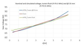
Figure 6: The RFQ voltage: nominal (red curve), tuner flush simulated (green curve), tuners at  $h_{t0} = 35 \text{ mm}$  (blue curve). The simulation was performed on 1/4 RFQ with 3 million mesh elements.
