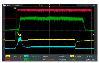
Figure 6: Stripping of Ar<sup>2+</sup> ions with the pulsed gas stripper. Shown are the current of the incoming beam (red) and the stripped Ar<sup>12+</sup> beam (green), voltage (yellow) and current (cyan) applied to the valve. Details see text.
