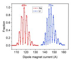
Figure 3: Xenon (red) and uranium (blue) charge state distributions after the liquid lithium stripper. The thickness is 1.05 mg/cm<sup>2</sup> for the xenon and 1.40 mg/cm<sup>2</sup> for uranium beams.
