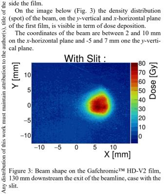
Figure 3: Beam shape on the Gafchromic™ HD-V2 film, 130 mm downstream the exit of the beamline, case with the
