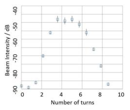
Figure 1: Stored beam intensity as a function of injection time with respect to the bumper trigger. One injection corresponds to one revolution time in the ring (one "turn"). The peak corresponds to ions which were efficiently injected, with the bumper voltage either too low or too high for proper injection outside of this region.
