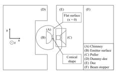
Figure 2: Top view of the SCALA source-puller model.
