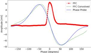
Figure 3: (Top) Snapshot of charge and field distribution measurements with FFC and PP within the macropulse. (Bottom) Averaged FFC and PP measurements along with convolution of FFC signal with impulse phase probe response.
