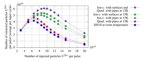
Figure 6: Results from simulations with cryogenic installations in the quadrupole and ion-catcher chambers at 15K with a cycle frequency of 2.7 Hz. More parameters are shown in Table 1.
