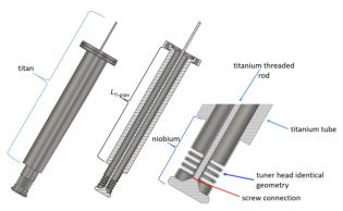
Figure 6: Bellow tuner adapted for tuner test bench.
