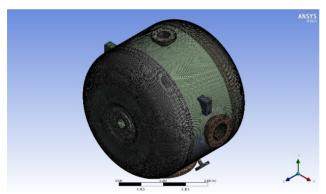
Figure 3: Mesh Shape of SSR2 SC cavity.
