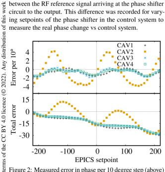
Figure 2: Measured error in phase per 10 degree step (above) and cumulative error from starting point of -220 degrees (below) vs setpoint in the control system.
