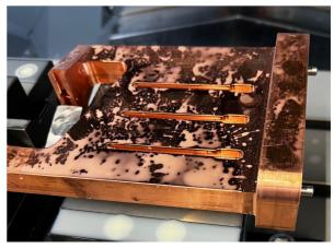
Figure 4: RFQ Stem during precision milling.
