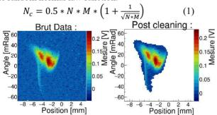
Figure 1: Before and after the matrix cleaning, with beam hotspots and tail, the extraction order is 9\*9 in this case.
