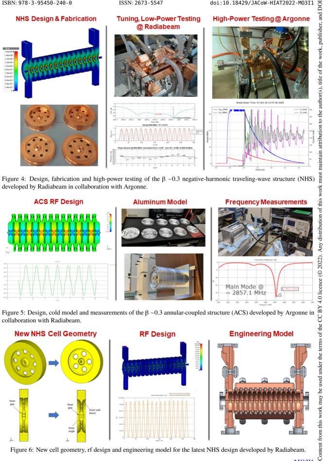
Figure 5: Design, cold model and measurements of the  $\beta \sim 0.3$  annular-coupled structure (ACS) developed by Argonne in collaboration with Radiabeam.
