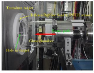
Figure 10: GTR measurements set-up
