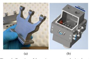
Figure 1: Overview of the cavity geometry and printed parts. (a) 3D printed girder drift tube structure. (b) Cross section of the assembled cavity model.
