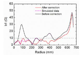
Figure 10: 1<sup>st</sup> harmonic amplitude ( $I_{\alpha} = 453$ A,  $I_{\beta} = 290$  A) before and after correction of large-hill-addition.
