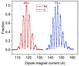
Figure 5: Xenon (red) and uranium (blue) charge state distributions after the liquid lithium stripper. The thickness is 1.05 mg/cm<sup>2</sup> for the xenon beam and 1.40 mg/cm<sup>2</sup> for the uranium beam.
