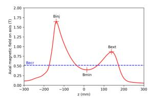
Figure 1: Typical 14 GHz ECRIS axial magnetic field profile on axis.
