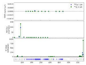
Figure 8: The signals from the beam loss monitors in the post-stripper section of the linac.
