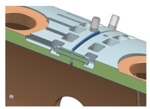
Figure 9: The inter-tank alignment detail: it is possible to recognise the slots for the bolts and the calibrated shims.
