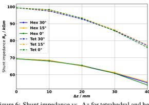
Figure 6: Shunt impedance vs.  $\Delta z$  for tetrahedral and hexahedral meshes at different  $\alpha$ .
