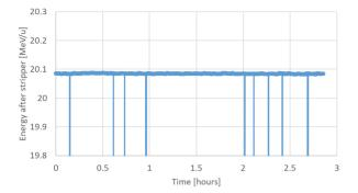
Figure 9: <sup>48</sup>Ca beam energy after the lithium stripper. At downward spikes the beam was tripped.
