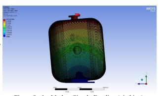
Figure 9: 1st Mode – Simply Bending (pitching).
