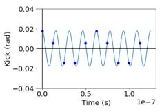
Figure 4: Average bunch deflection in the chopper due to the RF electric field overlaid onto a 64.4 MHz waveform.
