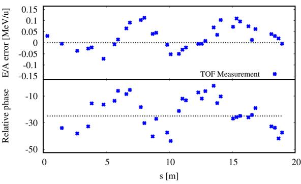
Figure 7: Measured energy and phase after each cavity of the test (blue) compared to expectations from the model (dashed line). X-axis is distance along the beamline.
