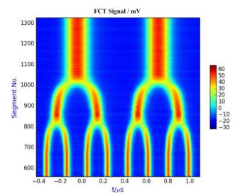
Figure 2: Waterfall plot of FCT signal after optimization of the two bunch merging sequences.
