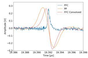
Figure 8: The FFC response convolved with the PP impulse response is much narrow in comparison to the PP signal.
