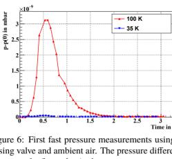
Figure 6: First fast pressure measurements using a piezo dosing valve and ambient air. The pressure difference with respect to the first value is shown.
