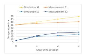
Figure 4: Measured and simulated temperatures at the respective measuring locations. The numbers increase with distance to the coldhead.
