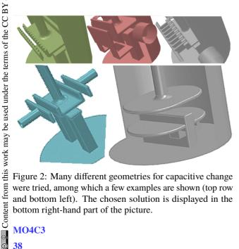
Figure 2: Many different geometries for capacitive change were tried, among which a few examples are shown (top row and bottom left). The chosen solution is displayed in the bottom right-hand part of the picture.
