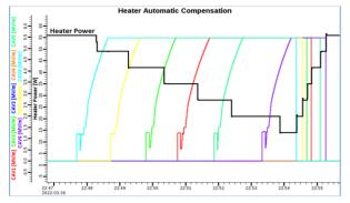
Figure 5: Cryo heater compensation based on cavity status.
