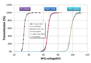
Figure 4: Transmission in the RFQ of the three reference Q/A.
