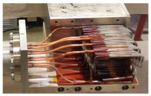
Figure 3: Septum coils with water supply (on the left) and the white insolation surface consisting of aluminum oxide.
