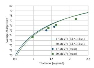
(b) Average charge states of uranium beam stripped by lithium
