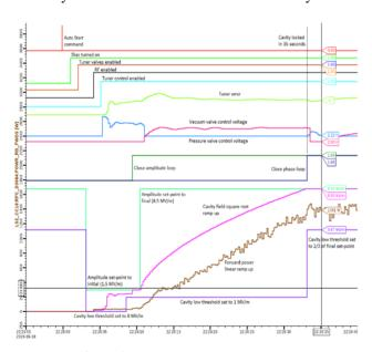
Figure 2: HWR auto turn on process.
