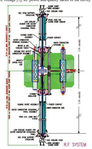
Figure 6: Half-wave coaxial RF cavity of SCC.
