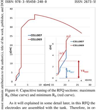
Figure 4: Capacitive tuning of the RFQ sections: maximum  $R_0$  (blue curve) and minimum  $R_0$  (red curve).
