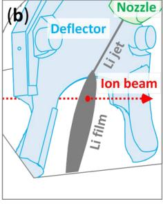
Figure 3: Liquid lithium charge stripper formed in a vacuum chamber which is part of the FRIB linac beamline. (a) Photograph of the lithium film and (b) sketch of what's seen in the photograph. A round jet of liquid lithium being issued from a nozzle impinges on a flat surface ("deflector"). The jet is then deflected forming a stable film that intercepts beams. The film is stable enough to have a mirror surface that reflects the surrounding components in the vacuum chamber or its inner wall.
