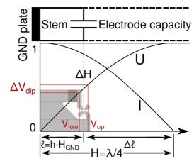
Figure 1: Potential distribution along the height of the stem. Showing the voltage difference between the upper and lower electrode pair [1].
