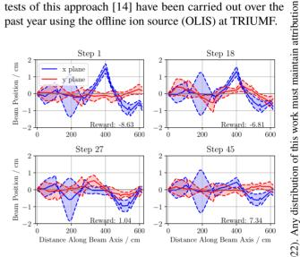
Figure 9: A validation of a trained agent on the simulated OLIS beam line. The panels show the evolution of the steerer predictions of a trained agent for different steps. The reward (calculated from the beam transmission) is increasing during the optimization process.
