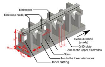
Figure 2: New type 4-rod RFQ model. This particular model uses a  $\Delta z = 20 \,\mathrm{mm}$  with  $\alpha = 15^{\circ}$ .
