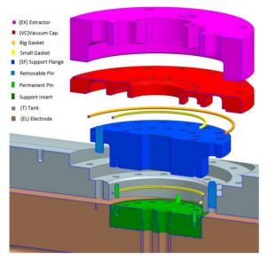
Figure 8: The assembly-alignment interface between electrodes and tank.
