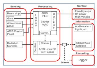
Figure 1: Schematic overview of the ARIS computer-PLC network.
