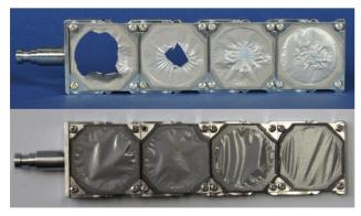
Figure 9: Foil ladders used during the 2010 low energy foil stripper tests. The same foil stripper before (bottom) and after (top) high current operation. 11 kJ were deposited in the third foil from left without any observed influence on the beam parameters [17].
