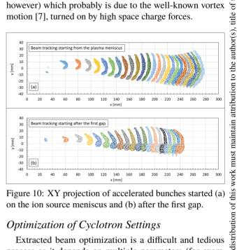
Figure 10: XY projection of accelerated bunches started (a) on the ion source meniscus and (b) after the first gap.
