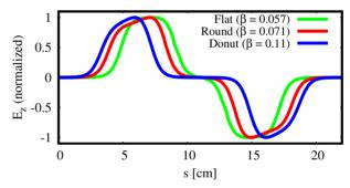
Figure 3: Normalized  $\mathcal{E}_z$  field maps of the three cavity types found in the ISAC-II linac.
