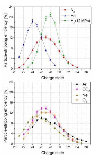
Figure 4: Charge state distributions for U stripped by N<sub>2</sub>, He and H<sub>2</sub> (top), Ar, CO<sub>2</sub>, Ne and O<sub>2</sub> (bottom), measured with the pulsed gas stripper at 1.4 MeV/u beam energy. The graphs show the equilibrium stripping efficiencies  $f_a$  as functions of the charge state q except for  $H_2$ , where the distribution was still not equilibrated at 12 MPa back pressure (from [12]).
