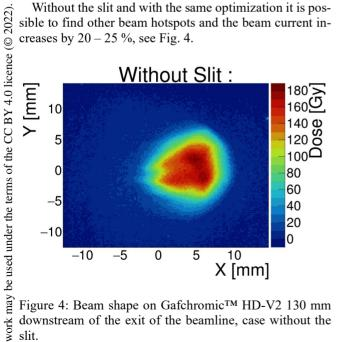
Figure 4: Beam shape on Gafchromic™ HD-V2 130 mm downstream of the exit of the beamline, case without the slit.
