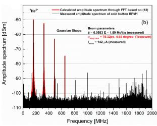
Figure 8: Comparisons between the calculated by Eq. (7) and the measured output voltage of cold button BPM1 in TD (a) and FD (b) during <sup>4</sup>He<sup>2+</sup> beam commissioning
