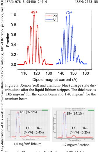
Figure 6: Charge state distributions of 20 MeV/u argon beam after the LLCS and carbon foil stripper. Thickness was 1.6 mg/cm<sup>2</sup> and 1.2 mg/cm<sup>2</sup> for the lithium and the carbon, respectively.
