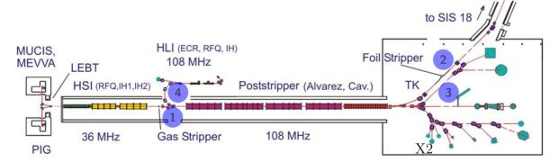
Figure 1: Schematic showing the UNILAC facility marking the location of various diagnostics. 1) Particle detectors 2) Dispersive section with RF deflector and screens 3) Gas Ionization BSM and 4) Feschenko BSM. R&D on FFC and GTR is ongoing in the area marked as "X2".
