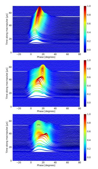
Figure 5: FFC bunch shape evolution for various single gap resonator phase (Top) 3 degrees, (Middle) 23 degrees and (Bottom) 43 degrees.
