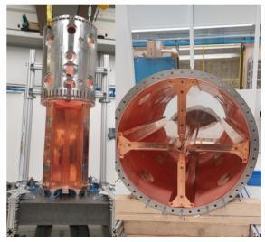
Figure 10: Initial positioning of Tank vs. electrodes (left), Final assembly of the RFQ module (right).
