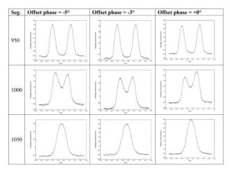
Figure 3: Optimization of 4:2 merging: FCT signal of two bunches merging into one (from top to bottom row) depending on the offset phase of the cavity with h = 2 (right column: default CCS settings with  $0^{\circ}$  offset).
