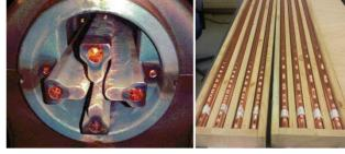
Figure 4: Installed HSI RFO electrodes after 10 years' operation (left); newly fabricated electrodes just before assembly (right).
