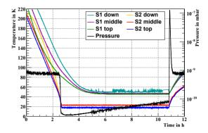
Figure 5: Temperature and pressure evolution during cooldown (0 h -  $2.5 \, h$ ), saturation measurement with hydrogen via dosing valve ( $2.5 \, h$  -  $11 \, h$ ), and the beginning of warmup (later than  $11 \, h$ ) with the fast pressure increase by the release of all adsorbed hydrogen. During saturation measurements, the lowest temperature sensor at stage one "S1 down" was subjected to distortions.
