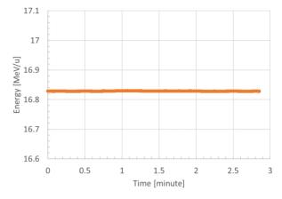
Figure 7: <sup>36</sup>Ar beam energy after the lithium stripper during the high-intensity irradiation test (peak intensity 12 particle uA, peak beam power 7400 W (average 400 W, duty cycle 5.4%), peak power loss 50 W (volumetric power deposition 6 MW/cm<sup>3</sup>).
