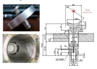
Figure 2: Button electrode, assembling picture and its drawing [4].
