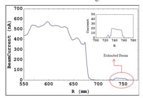
Figure 13: Beam current vs. radius for N<sup>2+</sup>, 4.5 MeV/u beam ( $f_{rf} = 14$  MHz, in 2<sup>nd</sup> harmonic mode of operation); First deflector entry was at 668.0 mm.
