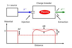
Figure 2: Electrostatic potential profile from the 1+ source to the ECR CB.
