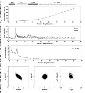
Figure 3: Simulation results for a carbon beam in the ACCIL linac up to 450 MeV/u. work may
