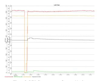
Figure 3: RFQ fast recovery after an s11 trip.
