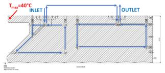
Figure 7: Cooling channel arrangement for the RFQ (case of high energy RFQ end).
