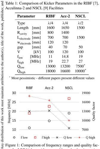
Figure 1: Comparison of frequency ranges and quality factors for 3 RF-kickers with comparable goals, showing a nice match to the trend of the Acculinna-2 kicker.
