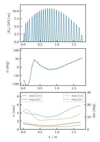
Figure 3: Gap voltages (top), synchronous phases (center) and resulting longitudinal and transverse beam envelopes (bottom) along Cavity-2.
