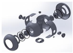
Figure 1: Layout of SSR2 Dressed Cavity.
