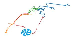
Figure 1: Layout of TRIUMF beamlines based on data from acc xml files. E-linac devices are shown in orange, primary proton beamlines in red, the new ARIEL RIB transport beamlines in green, and ISAC RIB transport beamlines in blue.
