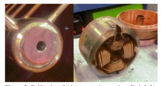
Figure 2: Drift tube of Alvarez section, as installed (left); opened drift tube with defective quadrupole lens (right).
