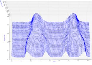
Figure 4: Mountain range plot of the FCT signal for the optimized 8:4 merging (segments 700 to 900) with phase offset  $+25^{\circ}$  for the ferrite cavity with h = 8.
