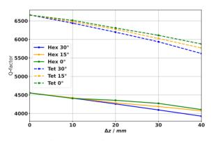
Figure 8: Q-factor vs.  $\Delta z$  for tetrahedral and hexahedral meshes at different  $\alpha$ .
