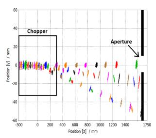
Figure 6: CST Studio simulation of the trajectory of bunches through the chopper, drift space, and the aperture.
