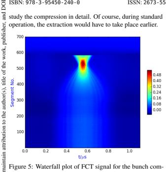
Figure 5: Waterfall plot of FCT signal for the bunch compression with extraction near segment 600. Each segment corresponds to one revolution period ( $T_R = 1.1 \mu s$ ).
