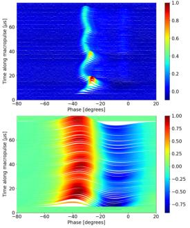
Figure 7: The waterfall plot showing the simultaneously recorded FFC and PP signal evolution along the macropulse A phase modulation along the macropulse is visible.
