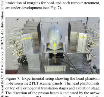
Figure 7: Experimental setup showing the head phantom in-between the 2 PET scanner panels. The head phantom sits on top of 2 orthogonal translation stages and a rotation stage. The direction of the proton beam is indicated by the arrow. The proton beam will be scanned vertically and horizontally with respect to this direction. The proton beam direction and entry point in the head phantom can be accurately controlled by combined translation and rotation of the phantom.
