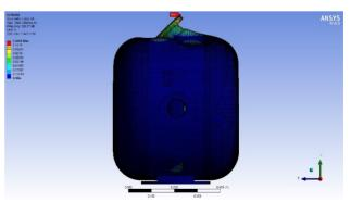
Figure 13: 5th Mode – Helium Outlet Bending.
