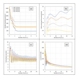
Figure 9: Beam rms properties, binned according to RF starting phase: (a) transmission, (b) beam centroid off-centering, (c) vertical beam size  $(2\sigma \text{ value})$ , (d) normallized vertical emittance ( $2\sigma$  value).
