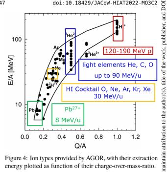
Figure 4: Ion types provided by AGOR, with their extraction energy plotted as function of their charge-over-mass-ratio.
