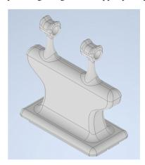
Figure 9: Improved geometry for the AM IH-structure.
