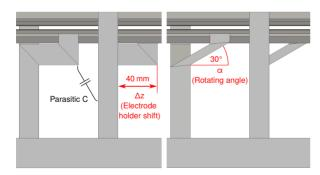
Figure 3: Side view of two variants of the model. Both variants use  $\Delta z = 40 \,\mathrm{mm}$  with  $\alpha = 0^{\circ}$  and  $30^{\circ}$ . Additionally depicted is the parasitic capacitance between one stem and the following stem.
