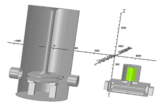
Figure 3: Soprano models of the conventional version using capacitive tuning (15-22 MHz) and of the version with saturable ferrite inductive tuning (15-45 MHz) are displayed on the same scale.
