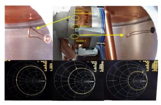
Figure 7: The coupler is rotated in 3 positions defined by the flange. Position 1 (left) gives a strong over-coupling, position 2 (mid) is still over-coupled and position 3 (right) is a bit under-coupled. The loop, in position 3, is then slightly deformed to increase its active surface and reach ideal coupling.
