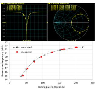
Figure 6: Factory tests results. Top pictures show the resonance peak (left) and Smith chart (right) at 22.539 MHz. At bottom measured and calculated values of the resonance frequency as a function of the distance between the bottom moving electrodes and their top counterpart.
