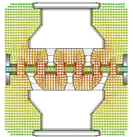
Figure 2: Electric field distribution in the prototype cavity.
