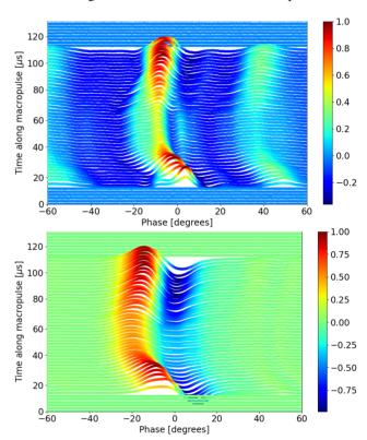
Figure 11: GTR and PP waterfall plot showing the bunch shape evolution along the macropulse.
