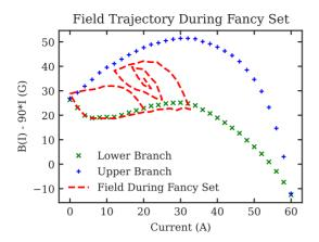
Figure 2: Field during algorithm for setting of magnetic quadrupoles.
