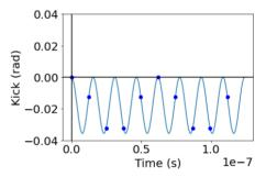
Figure 5: Average bunch deflection in the chopper due to the RF electric field combined with the static magnetic field provided by the chopper dipole overlaid onto a 64.4 MHz waveform.
