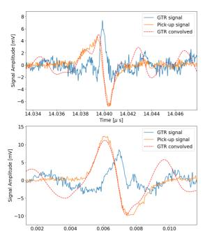
Figure 12: GTR signal along with its convolution through the PP response in comparison with the phase probe signal. A precise agreement between GTR and PP signal is seen.
