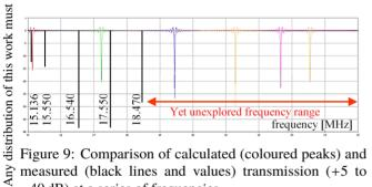
Figure 9: Comparison of calculated (coloured peaks) and measured (black lines and values) transmission (+5 to −40 dB) at a series of frequencies.
