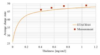
(a) Average charge states of xenon beam stripped by lithium.
