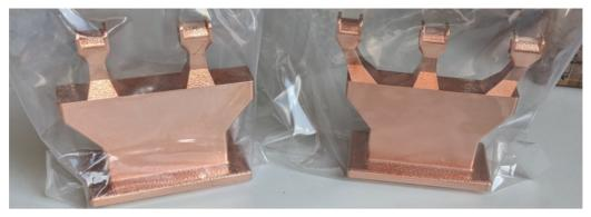
Figure 6: First iteration of AM stainless-steel IH-structures after polishing and galvanic copper-plating.
