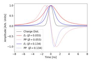
Figure 2: For the charge distribution ( $\sigma_t = 0.5 \text{ ns}$ ) showed by dashed lines, solid curves indicate the transverse field elongation for non-relativistic beam while dotted lines show the corresponding phase probe signal.
