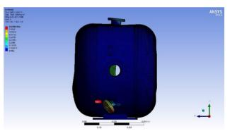
Figure 12: 4th Mode – Helium Inlet Bending.
