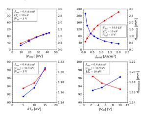
Figure 4: DC extracted current (red) and meniscus position (blue) as function of the four main parameters.
