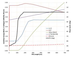
Figure 2: Main RFQ parameters vs length.
