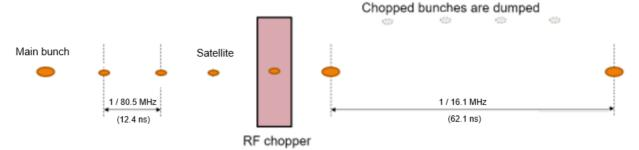
Figure 3: Bunch structure before and after the RF chopper system.
