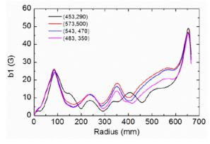
Figure 9: The 1<sup>st</sup> harmonic field amplitude vs. radius.
