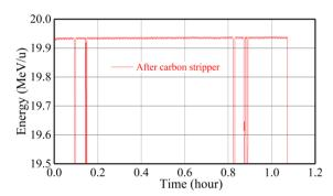
Figure 5: 82 Se beam energy after the stripper.
