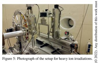
Figure 5: Photograph of the setup for heavy ion irradiations.
