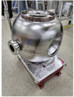
Figure 2: Fabricated SSR2 Bare Cavity.
