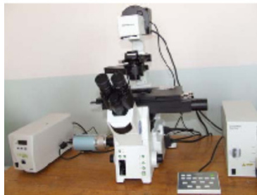
Inverted microscope for cell irradiation
