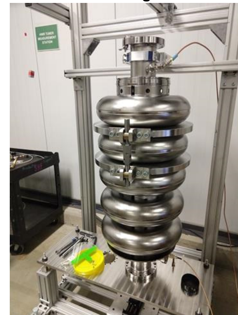
Field profile measurement after bulk EP, baking, and tuning
