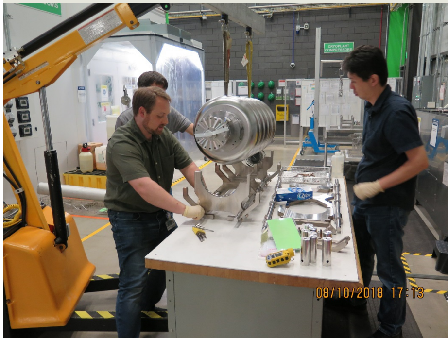
Dunk Test Insert for 644 MHz Upgrade Cavity
