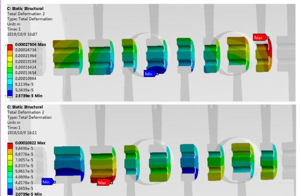
Fig.6: Without (above) and with (below) cooling system, the deformation distribution of drift tubes with 5/100 duty factor.
