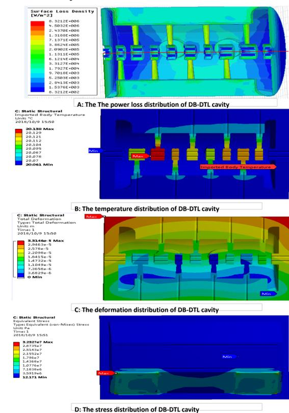
Fig.4: The power loss, temperature, deformation and stress distribution of the DB-DTL
