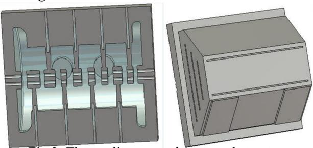
Fig.3: The cooling-water layout and structure model of the DB-DTL.
