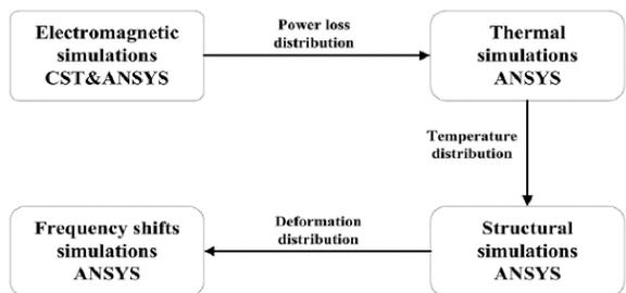
Fig.2: The multi-physics analysis scheme with MWS and ANSYS (Cited [6]).
