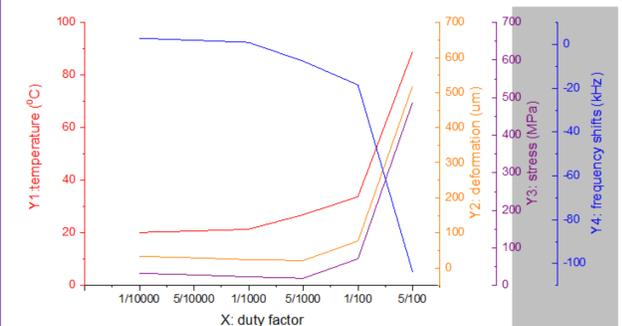
Fig.5: Without cooling-water system, the variation of the maximum cavity temperature, deformation stress and corresponding frequency shifts with duty factor.
