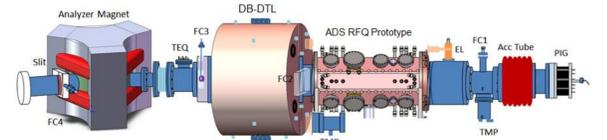
Fig.1: The layout of the DB-DTL beam test bench
